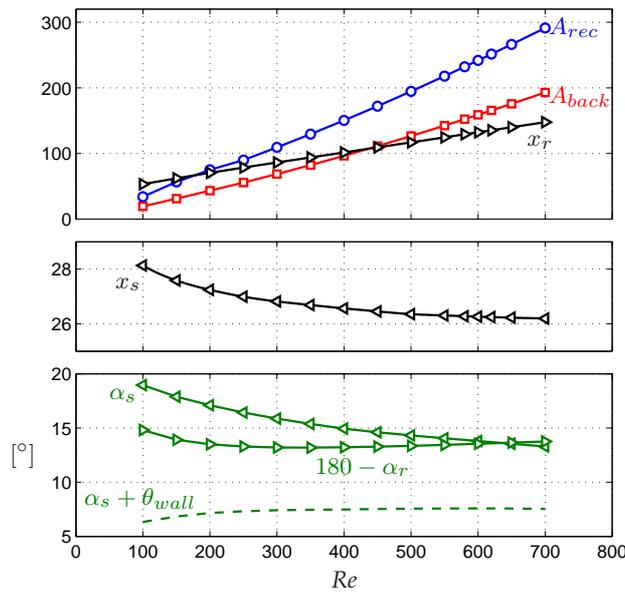
**Figure 4.** Variation with Reynolds number of characteristic separation quantities: recirculation and backflow areas  $A_{rec}$  and  $A_{back}$ , separation and reattachment locations  $x_s$  and  $x_r$ , separation and reattachment angles  $\alpha_s$  and  $\alpha_r$  relative to the wall (the dashed line shows the “absolute” separation angle  $\alpha_s + \theta_{wall}$ , i.e. measured relative to  $e_x$ ).
