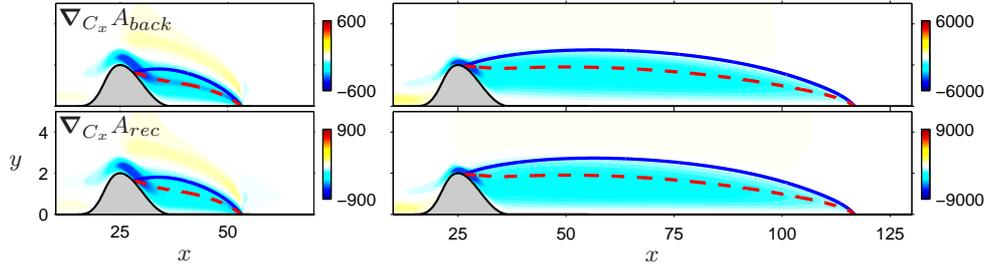
**Figure 8.** Sensitivity of backflow and recirculation areas  $A_{back}$ ,  $A_{rec}$ , with respect to streamwise volume control  $C_x$ . Left:  $Re = 100$ , right:  $Re = 500$ . The blue solid line is the separatrix, the red dashed line is the curve where  $U_x = 0$ .
