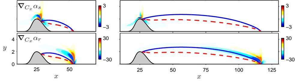
**Figure 7.** Sensitivity of separation and reattachment angles  $\alpha_s, \alpha_r$ , with respect to streamwise volume control  $C_x$ . Left:  $Re = 100$ , right:  $Re = 500$ . The blue solid line is the separatrix, the red dashed line is the curve where  $U_x = 0$ .
