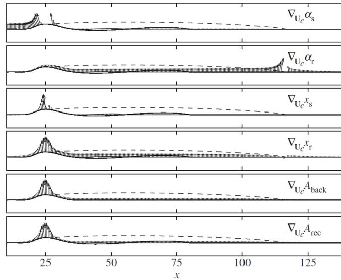
**Figure 10.** Sensitivity of separation and reattachment angles  $\alpha_s, \alpha_r$ , stagnation points  $x_s, x_r$ , backflow area  $A_{back}$  and recirculation area  $A_{rec}$  to wall control  $U_c$ . Arrows point in the direction of positive sensitivity. The dashed line is the separatrix.  $Re = 500$ .
