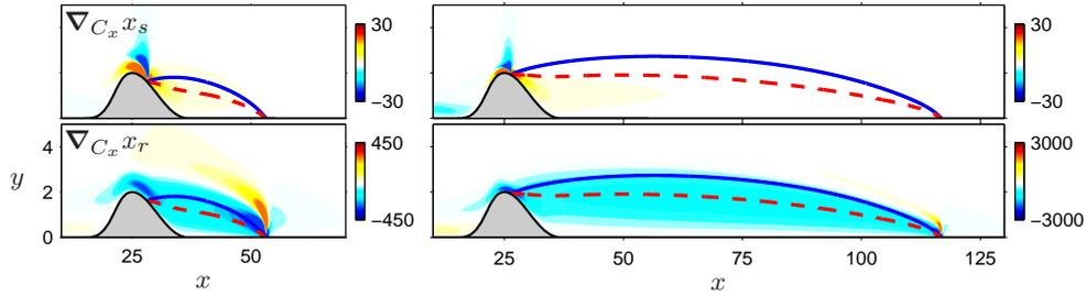
**Figure 6.** Sensitivity of stagnation points  $x_s$ ,  $x_r$ , with respect to streamwise volume control  $C_x$ . Left:  $Re = 100$ , right:  $Re = 500$ . The blue solid line is the separatrix, the red dashed line is the curve where  $U_x = 0$ .
