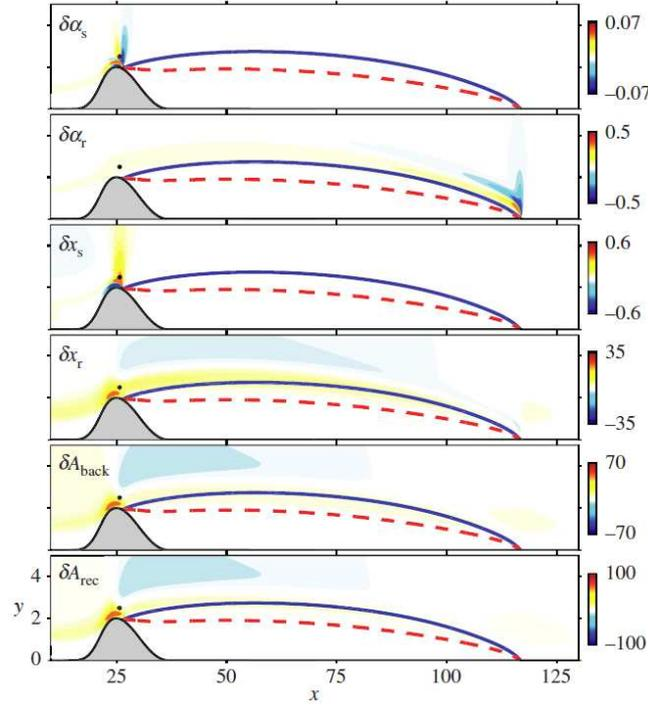
**Figure 9.** Effect of a control cylinder of diameter  $d = 0.05$  on separation and reattachment angles  $\alpha_s$ ,  $\alpha_r$ , stagnation points  $x_s$ ,  $x_r$ , backflow area  $A_{back}$  and recirculation area  $A_{rec}$ .  $Re = 500$ . The blue solid line is the separatrix, the red dashed line is the curve where  $U_x = 0$ . The black dot shows the position of the control cylinder  $(x_c, y_c) = (25.7, 2.5)$  used for validation in section 5(b).
