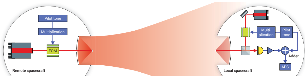
Figure 10. Pilot tone distribution for a single link of the observatory. At the remote spacecraft, the pilot tone frequency is multiplied and the signal is modulated onto the outgoing laser beam by an electro-optic phase modulator (EOM). A separate pilot tone on the local spacecraft is modulated onto the local laser to compare the two pilot tones in the sideband beat note of the heterodyne signal. To suppress the influence of ADC timing jitter, the local pilot tone is added to the heterodyne signal and used as a reference.
