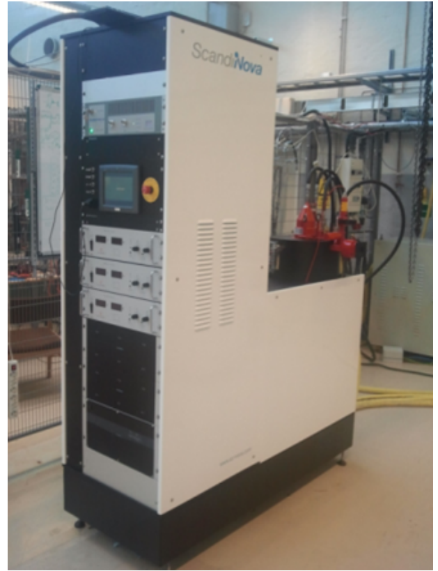
FIG. 24: Photograph of the compact RF transmitter that provides all power to photoinjector and linac.
