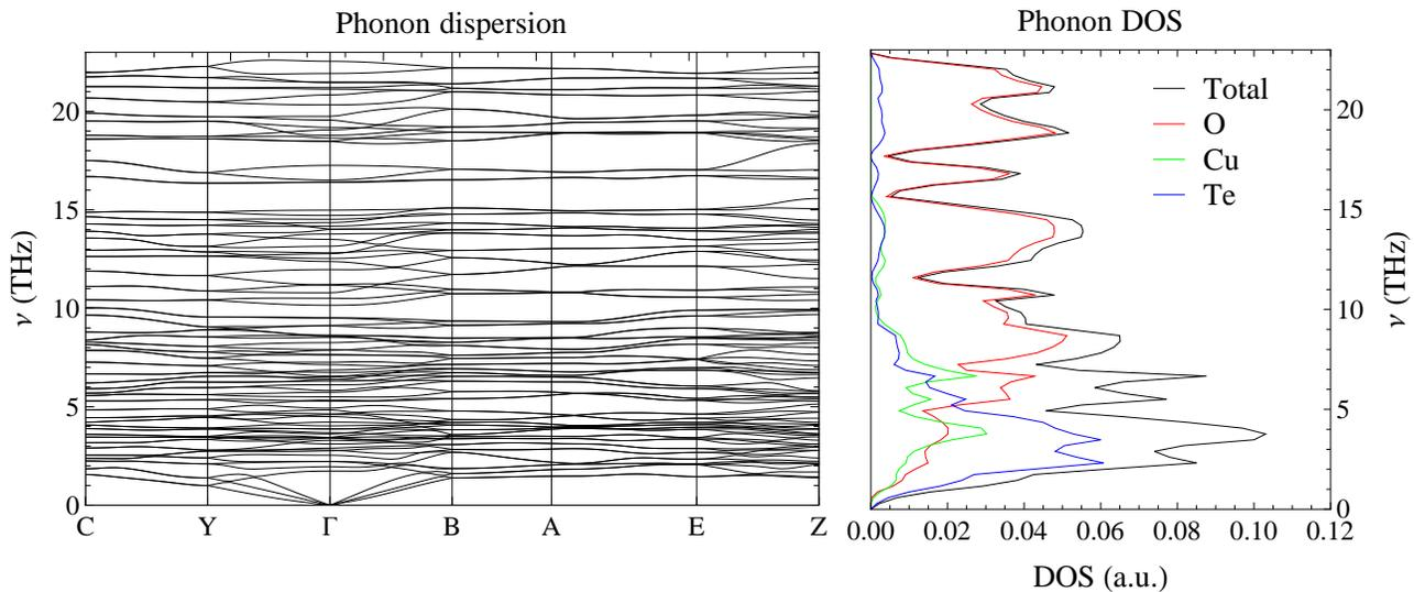
FIG. 2. Phonon dispersion and density of states, projected onto Cu, Te and O atoms for crystalline  $\text{CuTe}_2\text{O}_5$ .
