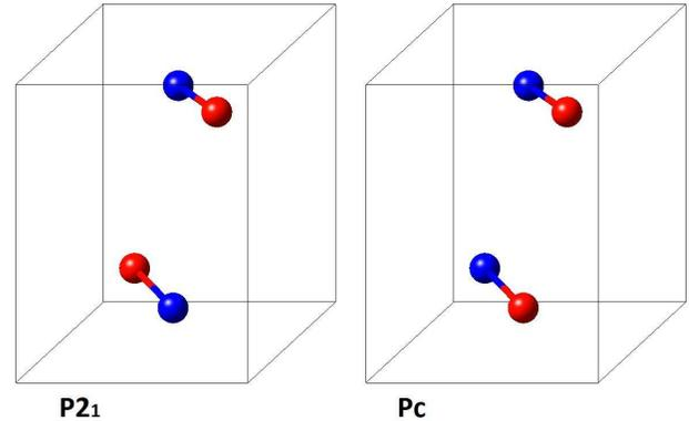
FIG. 1. The scheme of magnetic order of Cu-Cu structural dimers for two different symmetry subgroups ( $P2_1$  and  $Pc$ ) of space group  $P2_1/c$ . Red and blue spheres corresponds to the copper ions with spin up and spin down correspondingly, the magnetic moments value is  $0.75 \mu_B$ .
