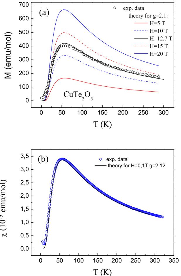
FIG. 5. Theoretically predicted temperature dependence of the magnetization (a) and magnetic susceptibility (b) of  $\text{CuTe}_2\text{O}_5$  for different values of the external magnetic field  $H$ . Open circles correspond to the experimental data (see text).
