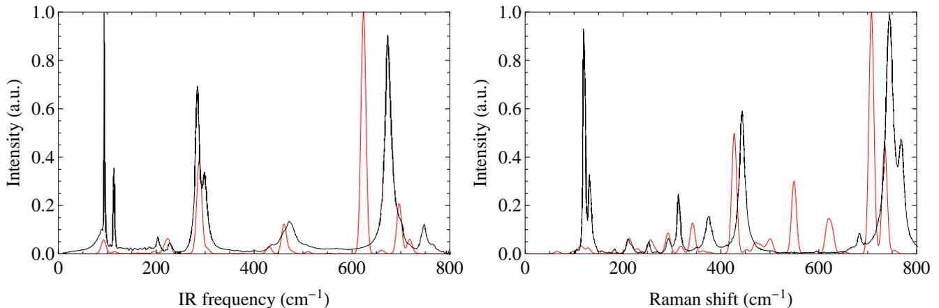
FIG. 3. Calculated (red) and experimental (black) [14] spectra for IR and Raman measurements, normalized to the maximum peak intensity. See text for details.
