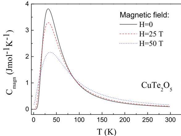
FIG. 6. Theoretically predicted temperature dependence of the magnetic contribution to the heat capacity of  $\text{CuTe}_2\text{O}_5$  for different values of the external magnetic field  $H$ .
