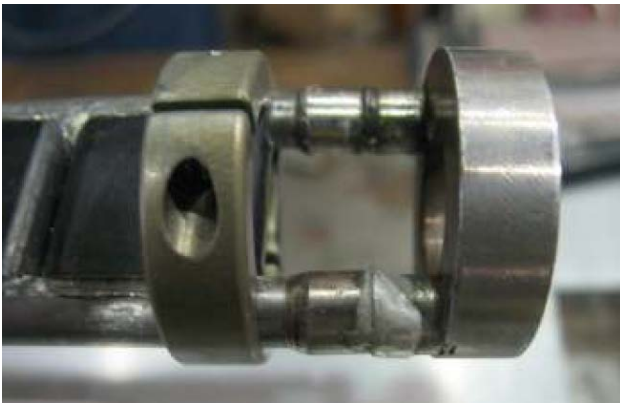
Figure 3: A downstream cooling water turn-around end of NuMI target NT-06 that failed after 4 month of operation at peak beam power of 340kW (total of 1.3 \times 10^{20} protons on target, 2011, courtesy J.Hylen, Fermilab)
