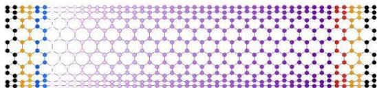
FIG. 1: Single-walled carbon nanotube under fixed boundary condition. Two layers (black atoms) from each side are kept fixed during the simulation. Blue (red) atoms are connected to the low (high) temperature thermostat. All the other atoms are simulated in the NVE ensemble. Dark purple indicates high mass region.
