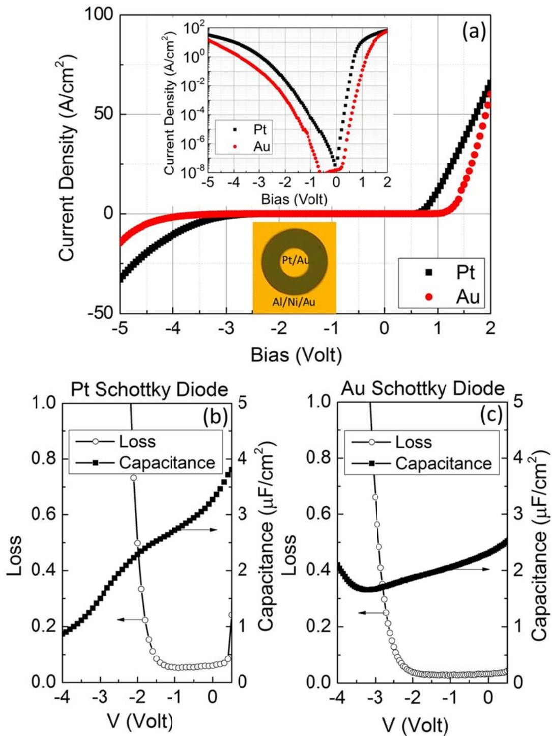
**Fig 1.** a) Measured I-V characteristics of Pt and Au circular Schottky diodes with 15  $\mu\text{m}$  radius (Inset: Optical image of the Pt Schottky diode), (b, c) Measured C-V characteristics (100 kHz, 30mV) of (b) Pt and (c) Au Schottky diodes.
