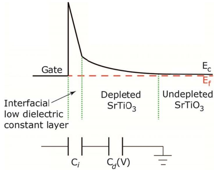
**Fig 4.** Schematic energy band diagram of a Schottky metal/SrTiO<sub>3</sub> junction showing the large voltage drop across the interfacial low dielectric constant layer and the effective capacitance model.
