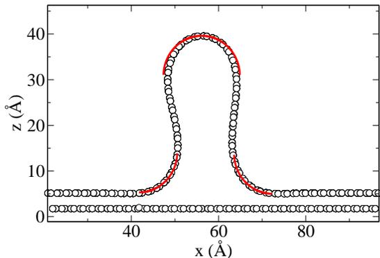
FIG. 7: Dots: the *standing fold* structure, as obtained in the simulations (also seen in Fig. 1(c)). Continuous curves: curvature radii as obtained from the analytical model, see Eq. (15) and relation (24).
