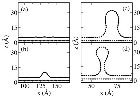
FIG. 1: Projection of the graphene bilayer into the  $xz$  plane obtained through simulations. (a) The moment immediately before the soliton formation at strain  $s = 2.8\%$  (see Sec. IV for the definition of the strain). (b) The soliton structure and (c) the structure we termed as *standing fold*, which appear at  $s = 27.5\%$ . (d) The structure which appear at approximately  $s = 28\%$ . We named it as *standing collapsed fold*.
