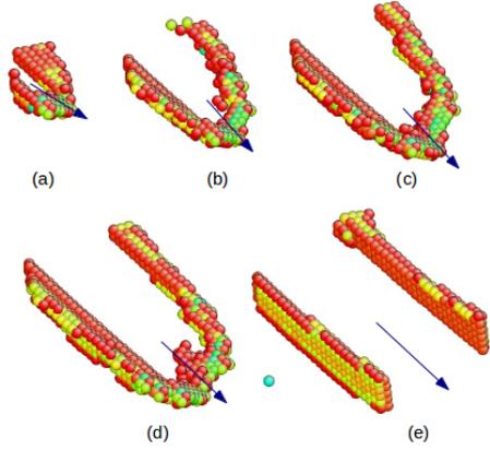
Figure 3: The typical mechanisms of straight screw dislocations pile-up in  $\langle 110 \rangle / \{111\}$  BCC Fe nanowires under tensile loading. The atoms on dislocation cores are only shown. The blue arrow represents the burger vector direction
