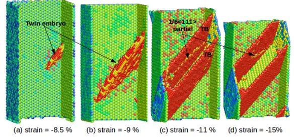
Figure 4: The atomic snapshots showing the deformation of  $\langle 110 \rangle / \{111\}$  BCC Fe nanowires under compressive loading. (a) The nucleation (b) growth of twin embryo (c) forming a full twin plate and (d) twin growth. The atoms are coloured according to the centro-symmetry parameter (CSP) [12]. The perfect BCC atoms and front surfaces are removed for clarity.
