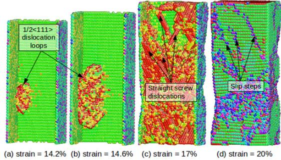
Figure 2: The atomic snapshots showing the deformation behaviour of  $\langle 110 \rangle / \{111\}$  BCC Fe nanowires under tensile loading. (a) The nucleation (b) expansion of dislocation loops (c) accumulation of straight screw dislocations and (d) the slip steps formed due to dislocation escape. The atoms are colored according to the centro-symmetry parameter (CSP) [12]. The perfect BCC atoms and the front surfaces are removed for clarity in (a-c).
