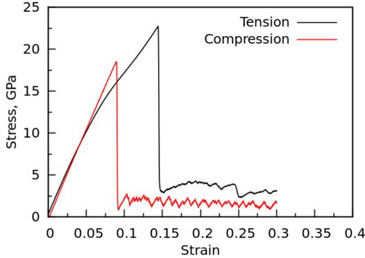
Figure 1: The stress-strain curves of  $\langle 110 \rangle / \{111\}$  BCC Fe nanowires at 10 K under tensile and compressive loading
