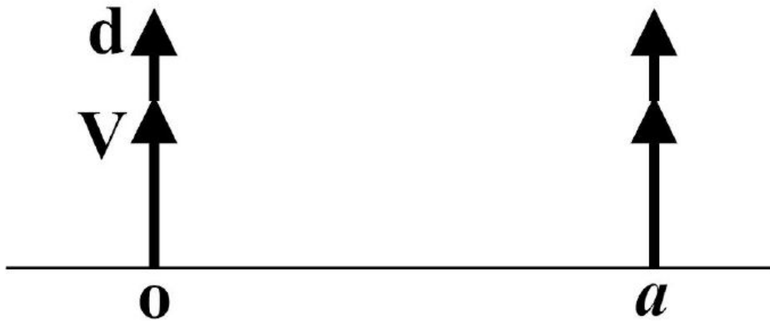
Figure 4: Kronig-Penney model with delta-function potentials. d is a perturbation, analogous to the self-energy potential V_S of 3D crystals.
