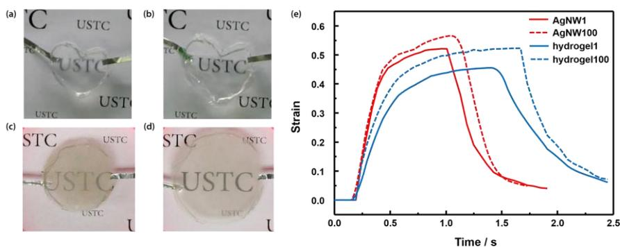
**Fig. 2. DEAs fabricated from hydrogel and AgNW compliant electrodes.** The initial (a) and activated (b) state of actuators based on heart-like PVA hydrogel. The initial (c) and activated (d) state of actuators based on circular
