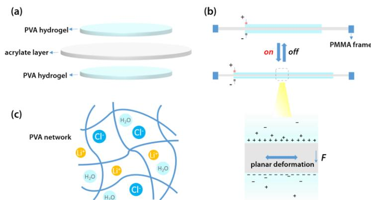
**Fig. 1. Schematic of dielectric elastomer actuator with compliant PVA hydrogel electrodes.** (a) A sandwiched structure. (b) Principle of reversible DEA actuation, and electrical double layer formed at the hydrogel-dielectric interfaces. (c) Illustration of ionic PVA network inside hydrogel electrodes.
