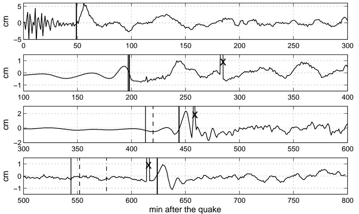
Figure 2: De-tided records of the Peruvian 08/2007 tsunami at DART buoys (top to bottom) 32401, 32411, 51406, 46412. Vertical lines mark the arrival of the front of the WMH (thick solid line), its estimate with the first buoy record for the next three buoys (thin solid), its estimate with the first and second buoy records for the next two buoys (dashed), its estimate with the three buoys for the last one (dashdot). Crosses mark trigger pulses (signals send by an operator).
