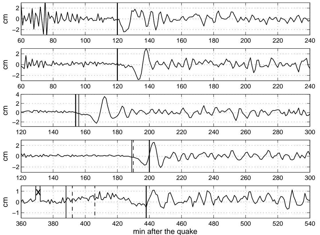
Figure 3: De-tided records of the Kuril 01/2007 tsunami at DART buoys (top to bottom) 21413, 21414, 46413, 46408, 46419. Vertical lines mark the arrival of the front of the WMH (thick solid line), its estimate with the first and second buoy records for the next three buoys (thin solid), its estimate with the first three buoy records for the next two buoys (dashed), its estimate with the four buoys for the last one (dashdot). Cross marks a trigger pulse (signals send by an operator).
