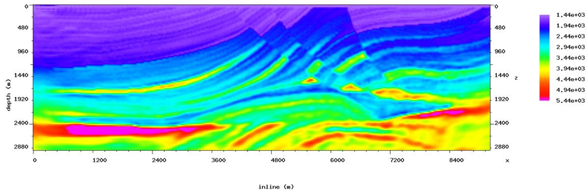
Figure 2: Baseline model inverted from noise-free synthetic data.
