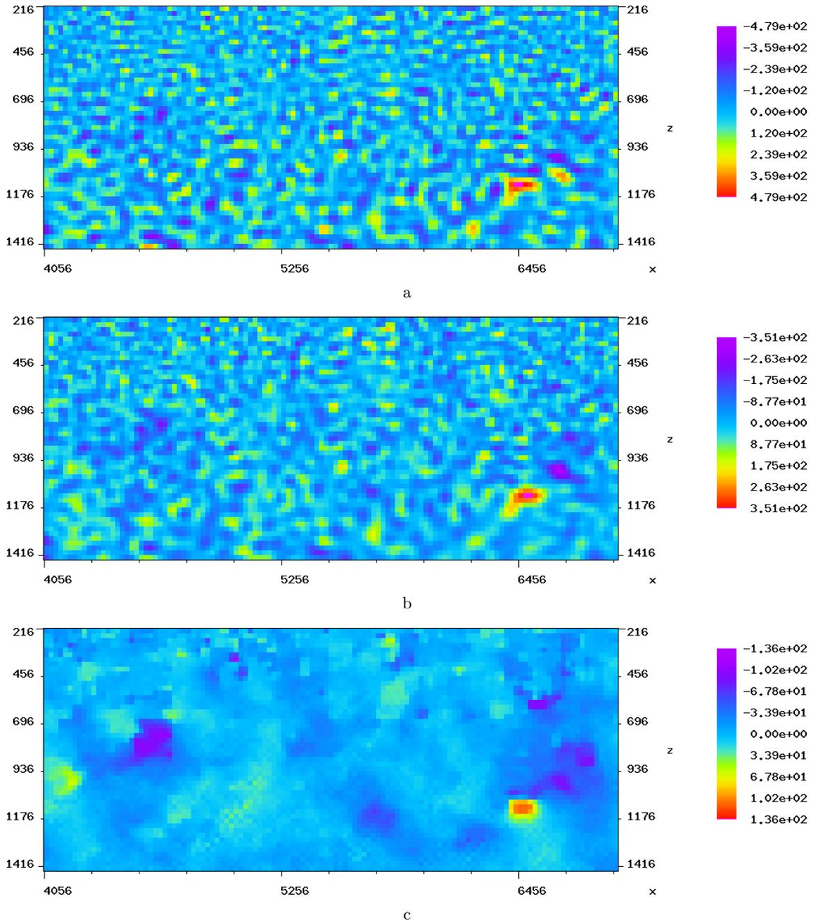
Figure 6: Model difference inverted from a 7 dB SNR synthetic with matching baseline and monitor acquisition geometries using (a) iterated parallel difference; (b) cross-updating; (c) regularized simultaneous inversion.
