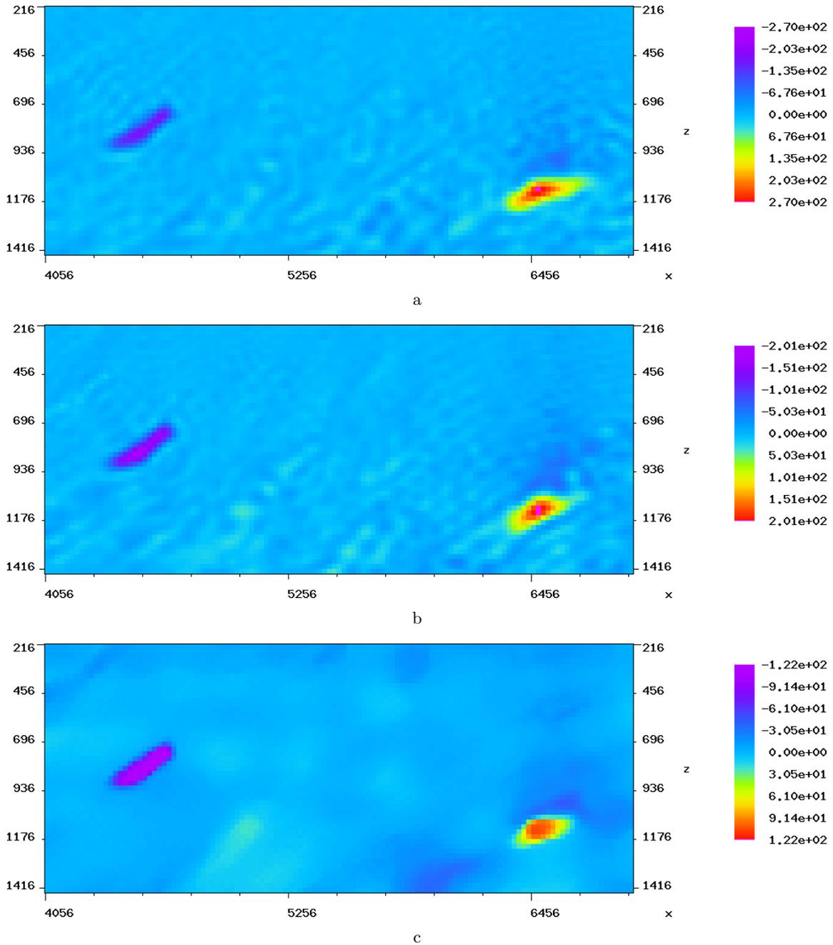
Figure 5: Model difference inverted from a clean synthetic with matching baseline and monitor acquisition geometries using (a) iterated parallel difference; (b) cross-updating; (c) TV-regularized simultaneous inversion.
