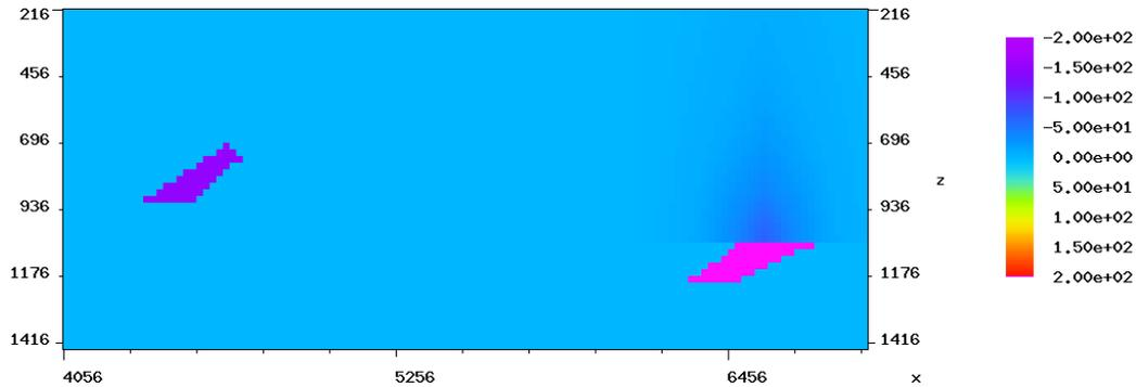
Figure 4: True velocity difference consists of a negative ( $-150$  m/s) perturbation at about 4.5 km inline 800 m depth, and a positive (200 m/s) perturbation at 6.5 km inline, 1 km depth.
