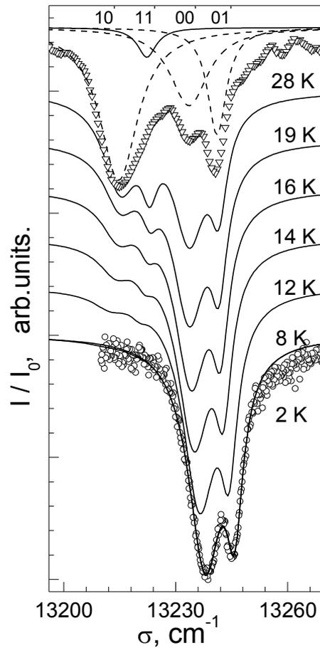
Figure 4. Evolution of the spectra based on the computing: transition  ${}^6\text{H}_{15/2} - {}^6\text{F}_{3/2}$ . Half-width of the initial doublet and additional two lines are linearly changed from its value at 2K. Summary intensity of the spectra is  $I_1+I_2$  for all temperatures, here  $I_1$  and  $I_2$  are intensities of the doublet components at 2K.
