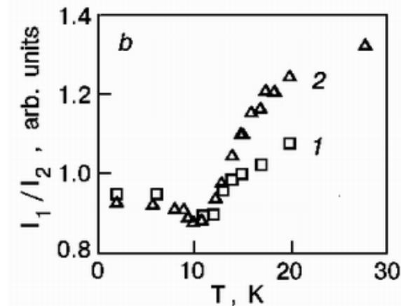
Figure 3. Ratio of intensities  $I_1/I_2$  for **E||c** (1) and **E||a** (2), here  $I_1$  and  $I_2$  are the relative intensities of the doublet components, transition  ${}^6F_{15/2} - {}^6F_{3/2}$ . For components 1 and 2 the ratio  $I_1/I_2$  is less than 1 for low temperatures.
