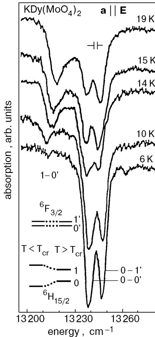
Figure 1. Temperature behaviour of the absorption spectra of KDy- molybdates at E||a polarisation of the light, transition <sup>6</sup>H<sub>15/2</sub>- <sup>6</sup>F<sub>3/2</sub> ; **a** is in the {010} plane. Scheme corresponds to the IR absorption spectra data for the one-ion representation.
