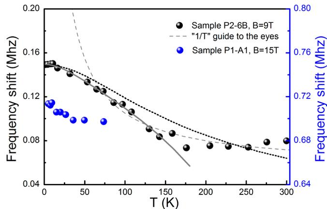
Figure S 7: Temperature dependence of the  $^{209}\text{Bi}$  frequency shift for samples P2-6B and P1-A1 at  $B = 9$  and  $15$  T, respectively. The dotted-line is the simulated variation of the shift using our 3DEG model (see text). The solid line further includes the effect of disorder. The dashed-line is a guide to the eyes for a  $1/T$  behavior.
