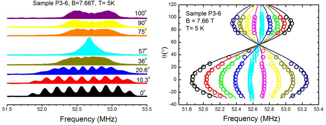
Figure S 4: Rotational pattern of the quadrupolar split  $^{209}\text{Bi}$  spectra at  $B = 7.66$  T and  $T = 5$  K. (a) Evolution of the spectra with the angle  $\theta$ . (b) Position of the resonances (open circles) obtained by fitting each spectrum with 9 Lorentzian functions, with proper constraints imposed by the spacing of the satellites. The solid lines are a fit of the angular dependence of the NMR spectrum with Eq. 11 (see text).
