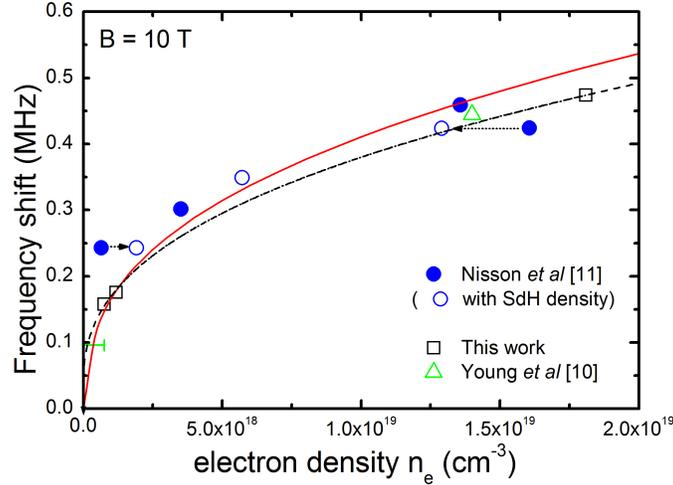
Figure S 6: Density dependence of the  $^{209}\text{Bi}$  central line shift for our samples, together with results obtained in other recent works. The horizontal dotted arrows show where the original data points are located when the electron density is estimated from SdH oscillations (see text). The solid line is the simulated variation of shift in the 3DEG model discussed in II.A. The dashed line is a fit to our data (black squares) allowing an extra non-zero intercept.
