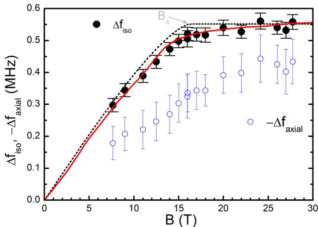
FIG. 3: (color online) Decomposition of the total frequency shift into isotropic ( $\Delta f_{iso}$ ) and axial parts ( $\Delta f_{axial}$ ) (see text) for sample P3-6. To compare the two components on the same graph,  $-\Delta f_{axial}$  is plotted. The black dotted line is a simulation in a 3D electron gas model ( $B_s$  indicates the field corresponding to full spin polarization). The red solid line further includes effects of the Landau quantization and of disorder.
