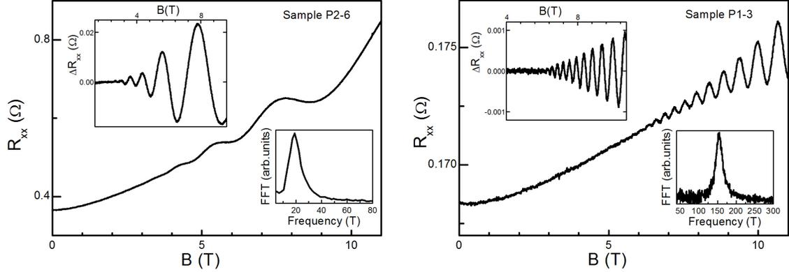
Figure S 1: Longitudinal resistance  $R_{xx}$  versus total magnetic field  $B \parallel c$ -axis for sample P2-6 (left panel) and P1-3 (right panel) at  $T=1.4$  K. Upper left insets: oscillatory resistance  $\Delta R_{xx}$ . Lower right insets: Fourier transform of  $\Delta R_{xx}(1/B)$ .
