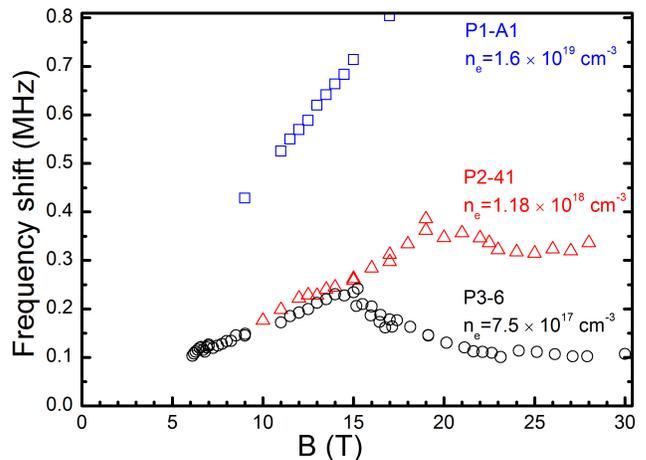
FIG. 2: (color online) NMR frequency shift ( $f - f_0$ ) of the Bi central line as a function of the magnetic field  $B$  applied along the  $c$ -axis, for three samples having different carrier concentrations.  $T = 5$  K.
