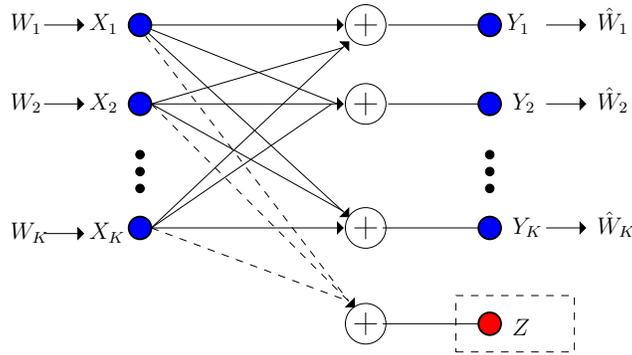
Figure 2:  $K$ -user interference channel (IC) with secrecy constraints.
