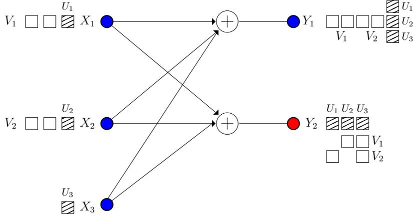
Figure 6: Illustration of secure interference alignment for the s.d.o.f. triple  $(\frac{2}{5}, \frac{2}{5}, 0)$  for the two-user MAC wiretap channel with one helper;  $K = 3$  and  $m = 2$ . Here, we define  $V_i \triangleq \{V_{ij} : j = 1, 2, 3, j \neq i\}$  for  $i = 1, 2$ .
