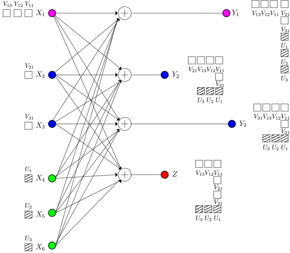
Figure 7: Illustration of secure interference alignment of Theorem 11 with  $m = 3, p = 2, N = 1$ .
