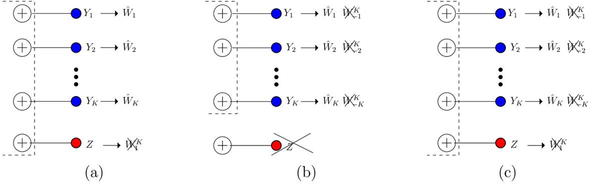
Figure 3: The receiver sides of the three channel models: (a)  $K$ -user IC-EE, (b)  $K$ -user IC-CM, and (c)  $K$ -user IC-CM-EE, where  $W_{-i}^K \triangleq \{W_1, \dots, W_{i-1}, W_{i+1}, \dots, W_K\}$ .
