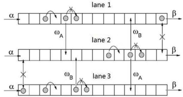
FIG. 1: Sketch of the three-lane TASEP. The arrow shows allowed hopping and the cross shows prohibited hopping.
