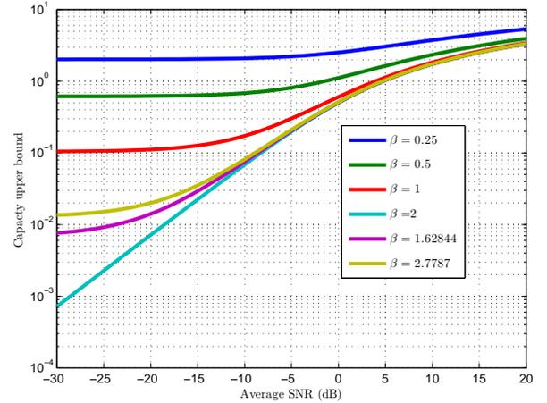
Fig. 3. The Capacity upper bound of AWGGN channel for different values of  $\beta$ .
