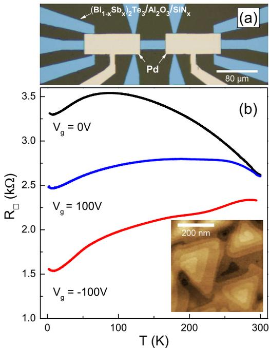
FIG. 1. (Color online) (a) Optical microscope image of the device. (b) Temperature dependences of  $R_{\square}$ , taken at  $V_g = 100$  V, 0 V and  $-100$  V. Inset: AFM image of a 20-nm-thick  $(\text{Bi}_{1-x}\text{Sb}_x)_2\text{Te}_3$  film capped with 4-nm-thick  $\text{Al}_2\text{O}_3$ .
