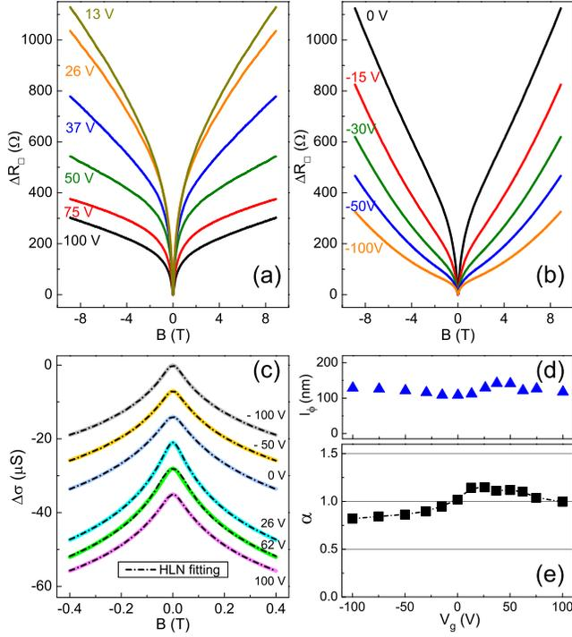
FIG. 3. (Color online) (a)-(b) Magnetoresistance at different gate voltages; (a) is for  $V_g \geq 13$  V and (b) is for  $V_g \leq 0$  V. (c) Magnetoconductance at representative  $V_g$  values; the curves are shifted vertically for clarity. The dashed-dotted lines are the fittings to Eq. (2). (d)-(e)  $V_g$  dependences of (d)  $l_\phi$  and (e)  $\alpha$  obtained from the fittings.
