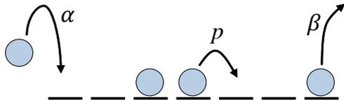
**Fig. 1** The TASEP with open boundaries. Particles come into the lattice from outside at the leftmost site with rate  $\alpha$ , hopping to the right with rate  $p$  under the exclusion interaction and getting out of the lattice from the rightmost site with rate  $\beta$ .
