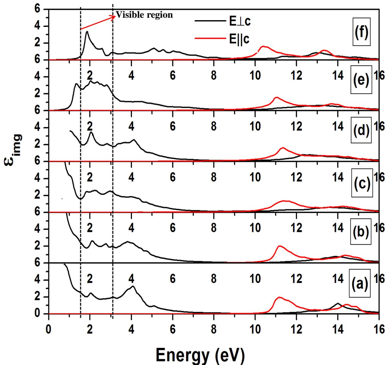
**Fig 6. The imaginary dielectric function for pure graphene (a) as compared with graphene sheet co-doped with different concentrations of BN in increasing order concentrations of boron in increasing order, 6.25% (b), 12.5% (c), 18.75% (d) and 37.5% (e) and 75% respectively for E<sub>⊥</sub>c and E<sub>||</sub>c.**
