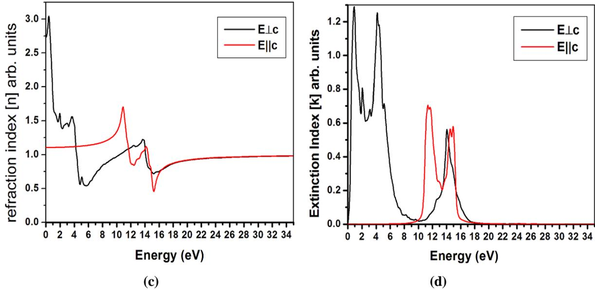
**Fig.3. The electron energy loss function (a), reflectivity (b), refraction index (c) and extinction index (d) of pure graphene for E $\perp$ c and E $\parallel$ c.**
