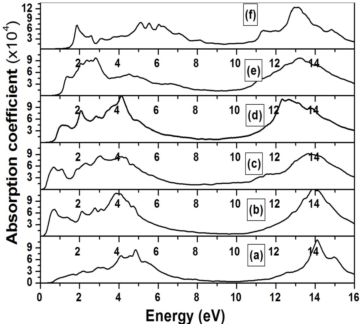
**Fig 10.** The absorption coefficient for pure graphene (a) as compared with graphene sheet co-doped with different concentrations of BN in increasing order concentrations of boron in increasing order, 6.25% (b), 12.5% (c), 18.75% (d) and 37.5% (e) and 75% respectively for E $\perp$ c.
