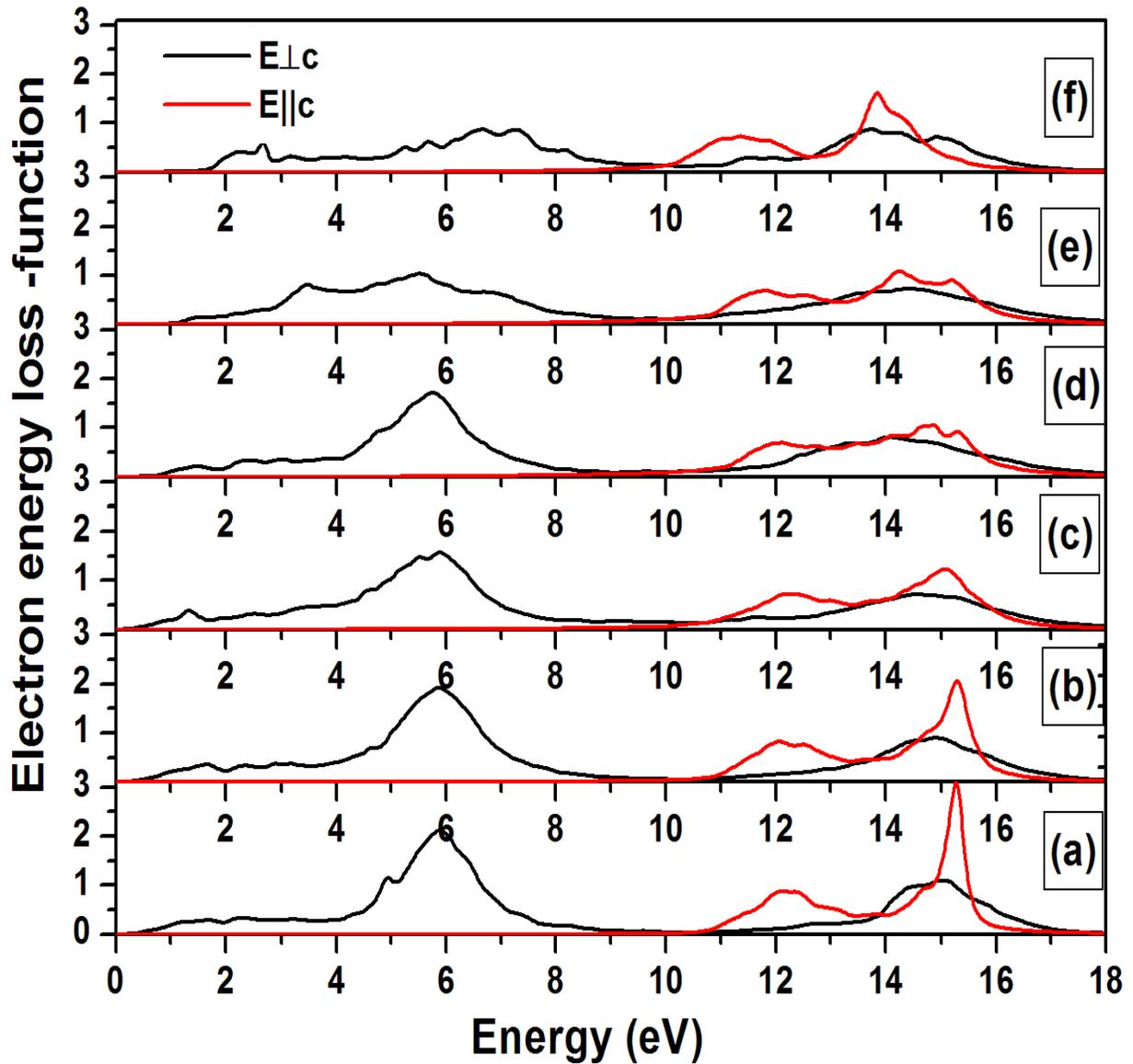
Fig 8 (b). The electron –energy loss spectra for pure graphene (a) as compared with graphene sheet co-doped with different concentrations of BN in increasing order concentrations of boron in increasing order, 6.25% (b), 12.5% (c), 18.75% (d) and 37.5% (e) and 75% respectively for  $E_{\perp c}$  and  $E_{\parallel c}$ .
