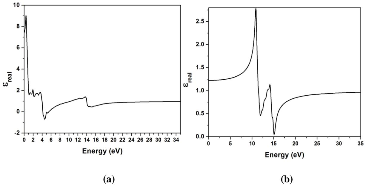
Fig.2. Real part of dielectric function of pure graphene for  $E_{\perp c}$  (a) and  $E_{\parallel c}$  (b)
