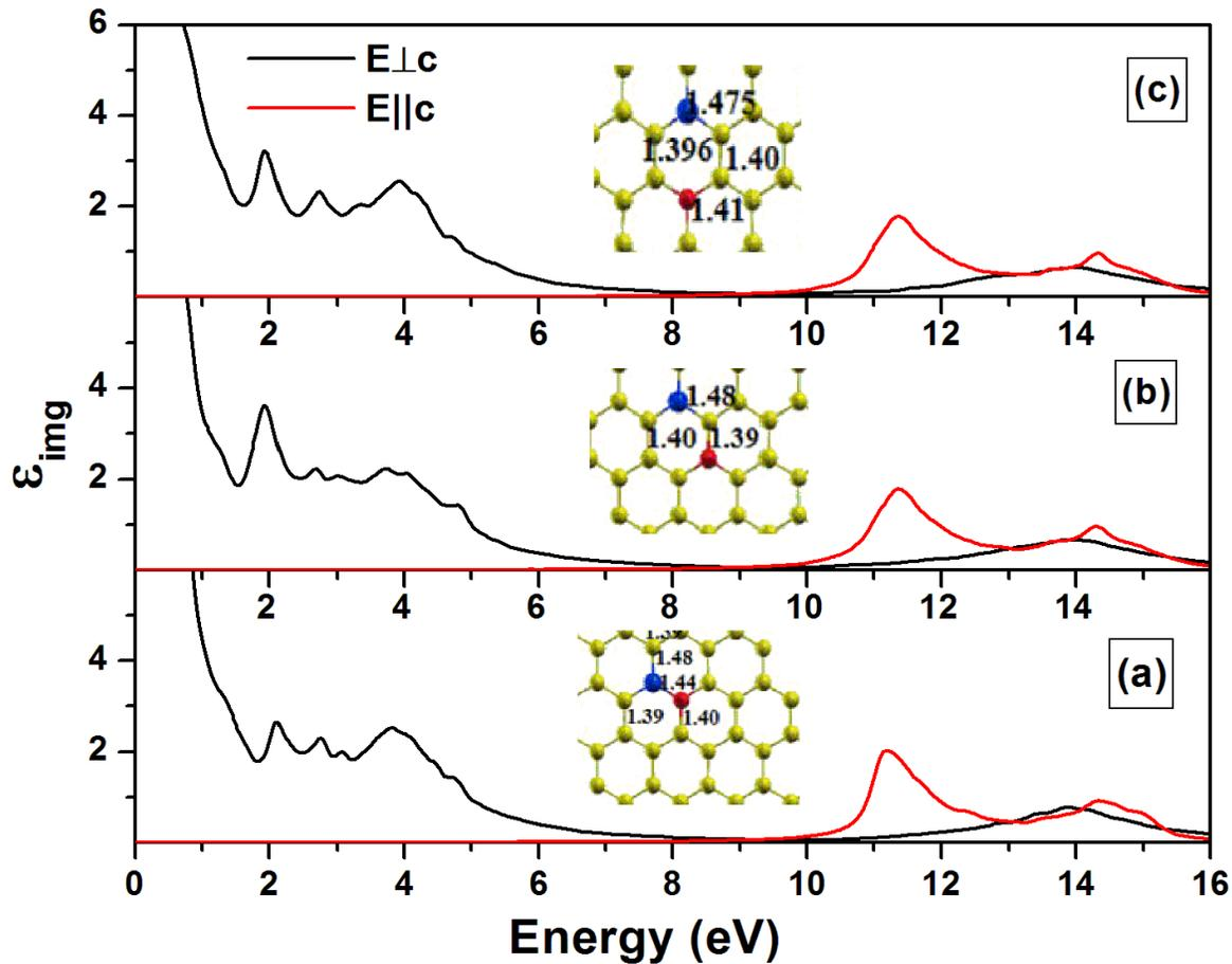
**Fig.7 (b).** Comparison of imaginary part of dielectric function of pure graphene with that of B/N co-doped graphene sheet for different doping sites, ortho (a), meta (b) and para isomer (c).
