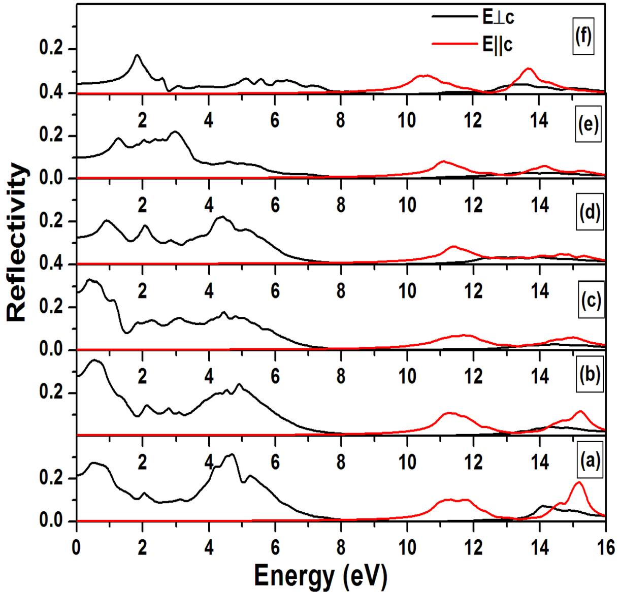
Fig 9. The reflectivity for pure graphene (a) as compared with graphene sheet co-doped with different concentrations of BN in increasing order concentrations of boron in increasing order, 6.25% (b), 12.5% (c), 18.75% (d) and 37.5% (e) and 75% respectively for  $E_{\perp c}$  and  $E_{\parallel c}$ .
