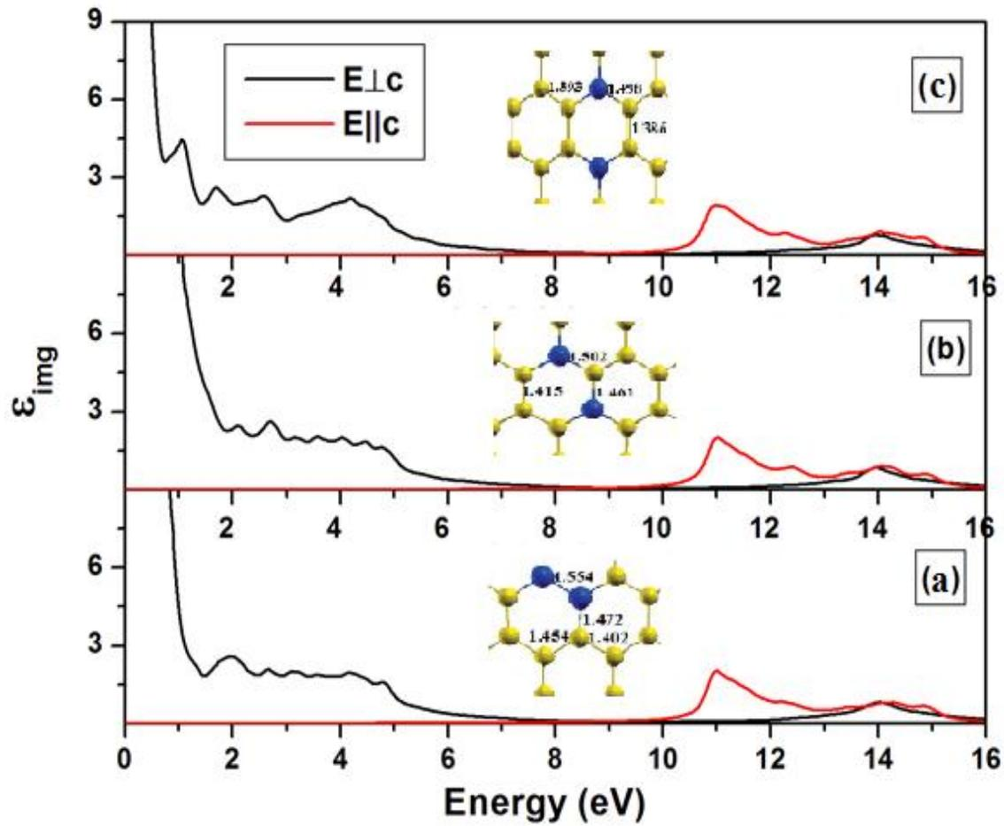
Fig.7 (a). Comparison of imaginary part of dielectric function of three different isomers of graphene sheet doped with 2 boron atoms with configurations as shown in inset for in-plane light polarization ( $E \parallel c$ ).
