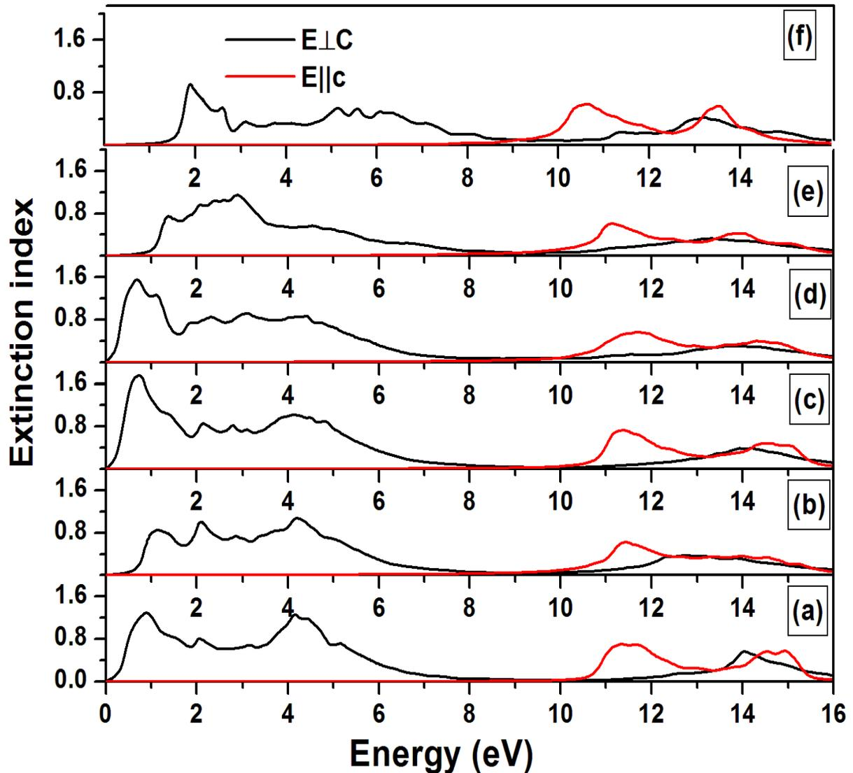
**Fig 11.** The extinction index for pure graphene (a) as compared with graphene sheet co-doped with different concentrations of BN in increasing order concentrations of boron in increasing order, 6.25% (b), 12.5% (c), 18.75% (d) and 37.5% (e) and 75% respectively for  $E_{\perp c}$  and  $E_{\parallel c}$ .
