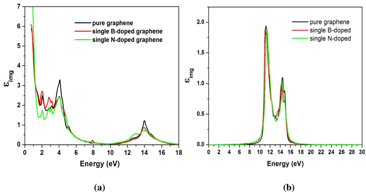
**Fig.4. Comparison of imaginary part of dielectric function of pure graphene with that of single boron and nitrogen atom doped graphene sheet for  $E \perp c$  (a) and  $E \parallel c$  (b).**
