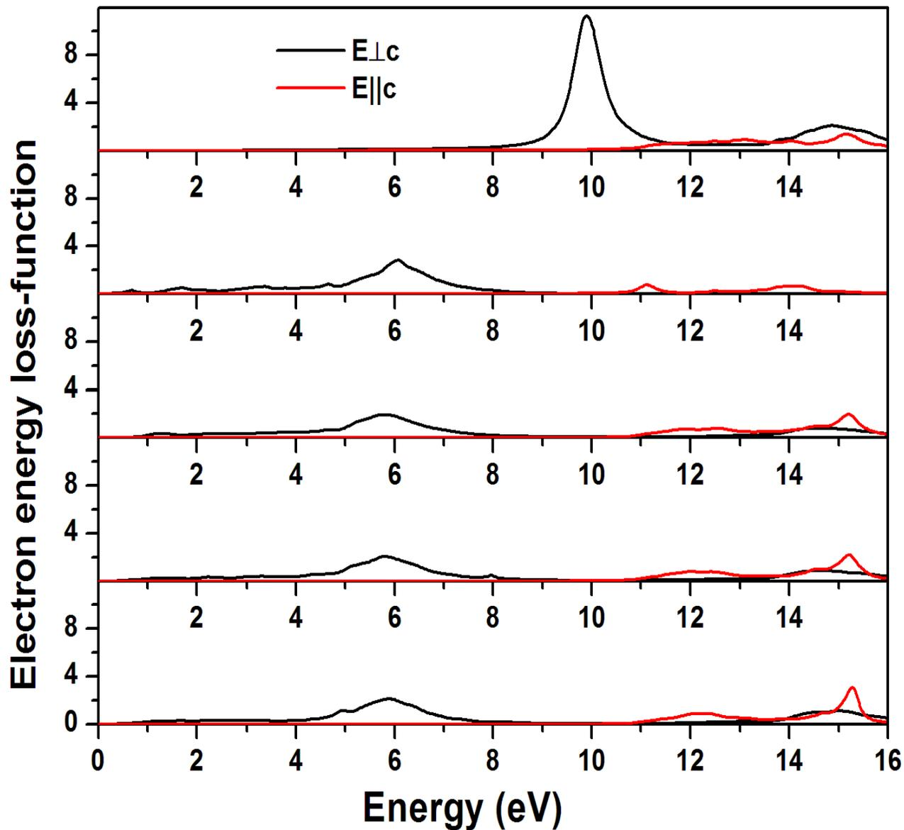
Fig 8 (a). The energy-loss function for pure graphene (a) as compared with graphene sheet doped with different concentrations of boron in increasing order (upwards), 3.125% (b), 6.25% (c), 9.375% (d) and 18.75% (e) respectively.
