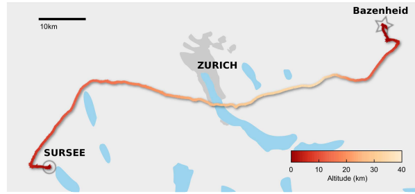
FIG. 4. Flight path of the helium balloon hosting the device under test. The balloon reached a maximum altitude of 35.5 km before bursting.
