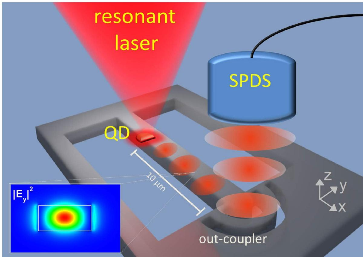
**Figure 1. Experimental scheme for observing QD resonance fluorescence in a waveguide.**
