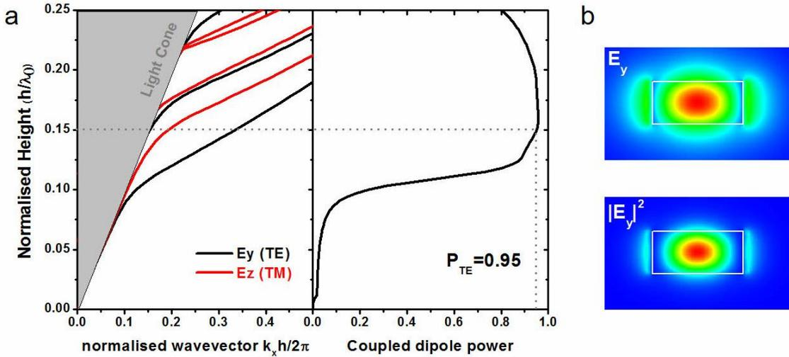
**Figure S2. Results of FDTD simulations of waveguide modes.** (a) Modes structure in a GaAs waveguide with an aspect ratio of 2. For a normalised height of  $h/\lambda_0=140/930=0.151$ , the waveguide fully sustains a single  $TE$  mode with 95% coupling. (b) Electric field and intensity profile of the first  $TE$  mode for  $h/\lambda_0=0.151$  and  $w=2h$ .
