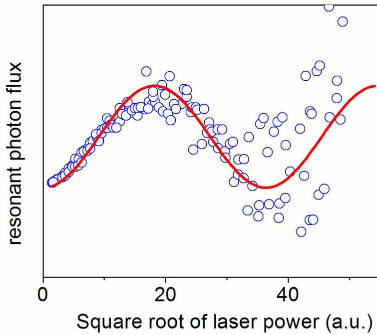
**Figure 5. Rabi oscillation in resonance fluorescence.**
