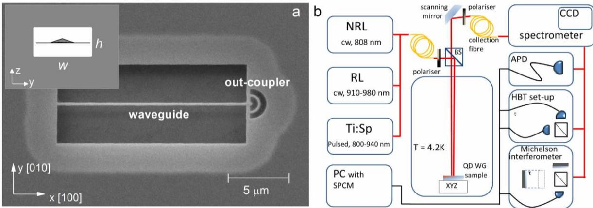
**Figure S1. Sample and Set-up.** (a) SEM image of the suspended GaAs single-mode waveguide with an out-coupler at one end. The Inset shows a schematic of the cross-section of the waveguide (WG) of height and width,  $h$  and  $w$ , respectively, with a quantum dot shown embedded at the centre. (b) Schematic diagram of the experiential set-up. RL – resonant laser, NRL – non-resonant laser, SPCM – single photon counting module.
