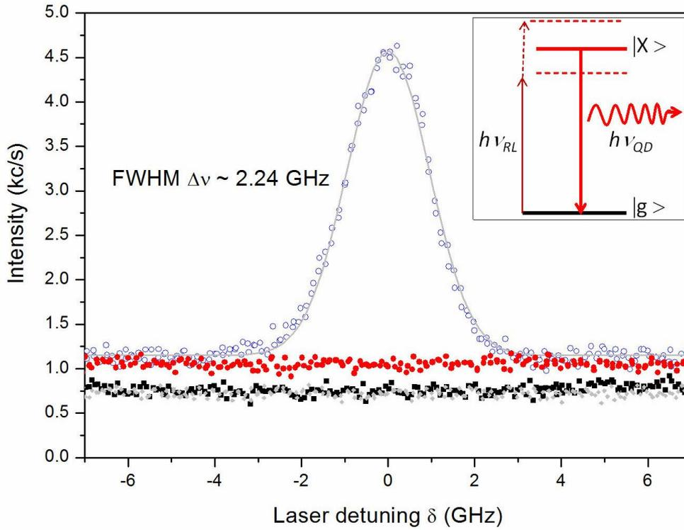
**Figure 2. QD resonance fluorescence with slow-scanning resonant laser.**
