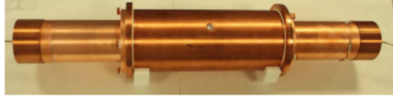
Figure 1: ANAIS-25:D0 module: 12.5 kg mass crystal by Alpha Spectra coupled to two PMTs (Hamamatsu R12669SEL2) at the LSC clean room. Calibration window can be noticed.
