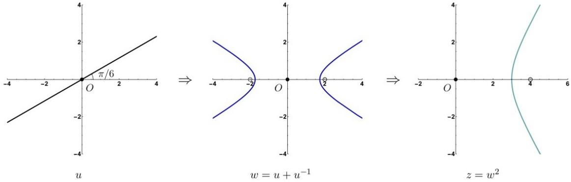
FIG. 3: The image of a **straight line** through the origin of the **u**-plane with inclination  $0 < \phi < \pi/4$  is a **Zhukovsky hyperbola**, whose centre is the origin of the **w**-plane. Squaring the latter provides us with the **right**-branch of a hyperbola in the **z**-plane, whose outer focus is  $z = 0$ .
