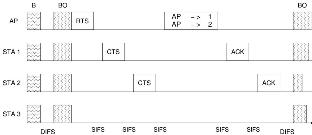
Fig. 11. A successful downlink MU-MIMO transmission
