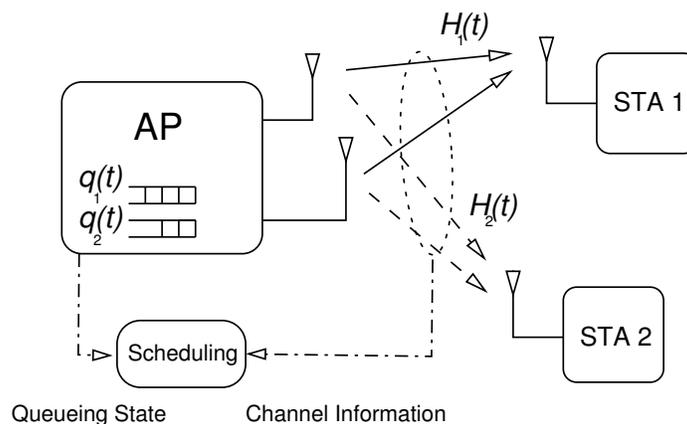
Fig. 7. Queueing and channel based cross-layer scheduling
