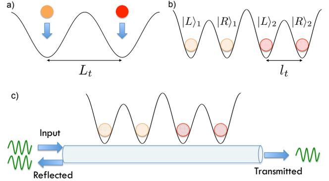
FIG. 1. (color online). Trapping and probing schemes in the case of two atoms in adjacent wells. (a) Simple-well configuration ( $A = 0$ ) with localized atoms (dark colors). (b) Double-well configuration ( $A \neq 0$ ) with atoms in a spatial superposition (light colors). (c) Probing of the atomic spatial state through the photon transmission and reflection spectra.
