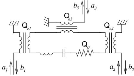
FIG. 3. Microwave cavity represented as three port device.
