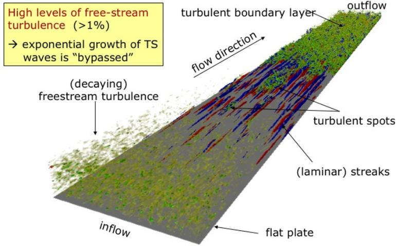
Fig. 6. Sketch of bypass transition in a boundary layer exposed to high levels of free-stream turbulence. Details of the simulations are reported in Brandt et al. (2004); Schlatter et al. (2008). Visualization courtesy of Philipp Schlatter.
