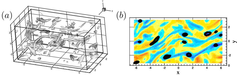
Fig. 9. (a) Snapshot of the quasi-streamwise vortices and (b) the associated vortex sheets during the early stages of the turbulent kinetic energy growth in a homogeneous shear flow (see also Gualtieri et al., 2002).
