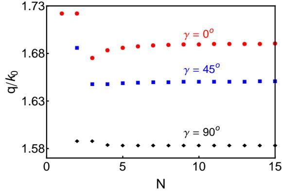
Figure 3: The wavenumbers  $q/k_0$  calculated as solutions of the surface-wave dispersion equation as a function of  $N \in [1, 15]$  and  $\gamma \in \{0^\circ, 45^\circ, 90^\circ\}$  for Dyakonov–Tamm waves guided by the interface of magnesium fluoride ( $\varepsilon_s = 1.896$ ) and an ambichiral dielectric material characterized by Eqs. (5) with  $\chi_v = 20^\circ$ . For these calculations, we fixed  $\lambda_0 = 633$  nm and  $\Omega = 200$  nm.
