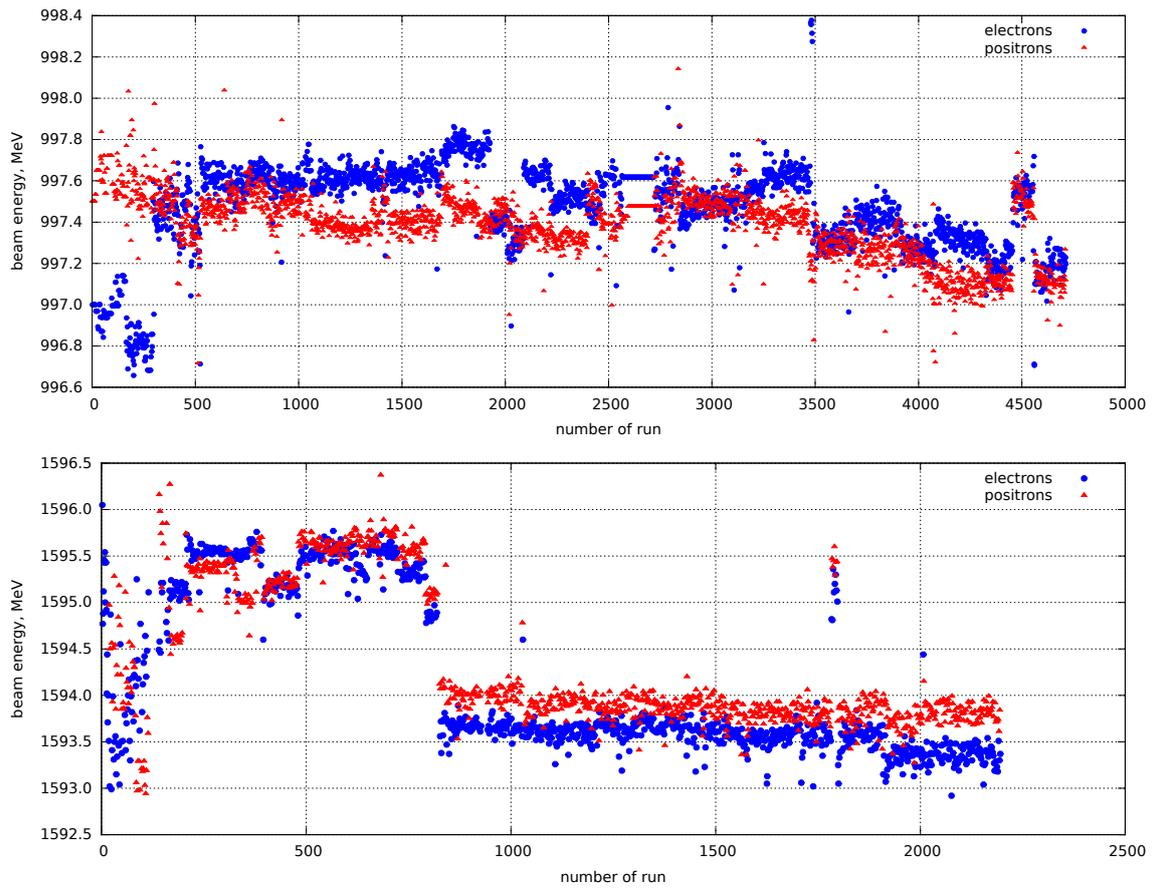
**Figure 9.** Measured beam energy versus run number (with electron or positron beam): top panel for the first phase of the experiment, bottom panel for the second one. The blue circles correspond to electron beams and the red triangles to positron beams.
