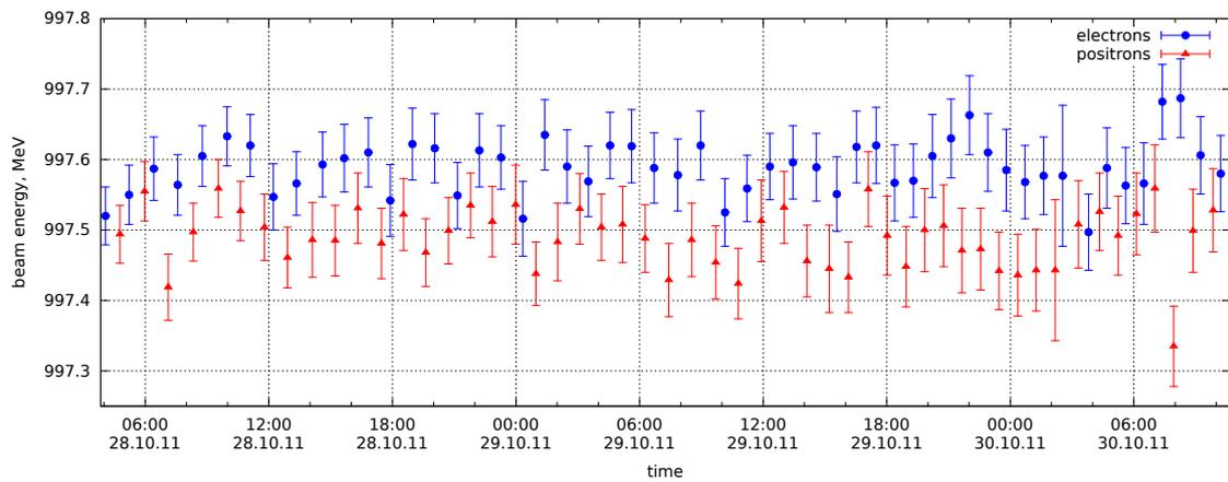
**Figure 10.** Short-term behaviour of the beam energy for the first phase of the experiment. The blue circles correspond to electron beams, and the red triangles to positron beams.
