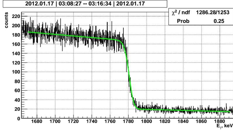
**Figure 8.** The Compton edge in the HPGe detector spectrum. It is fitted by a convolution of a step-like function with the response function.
