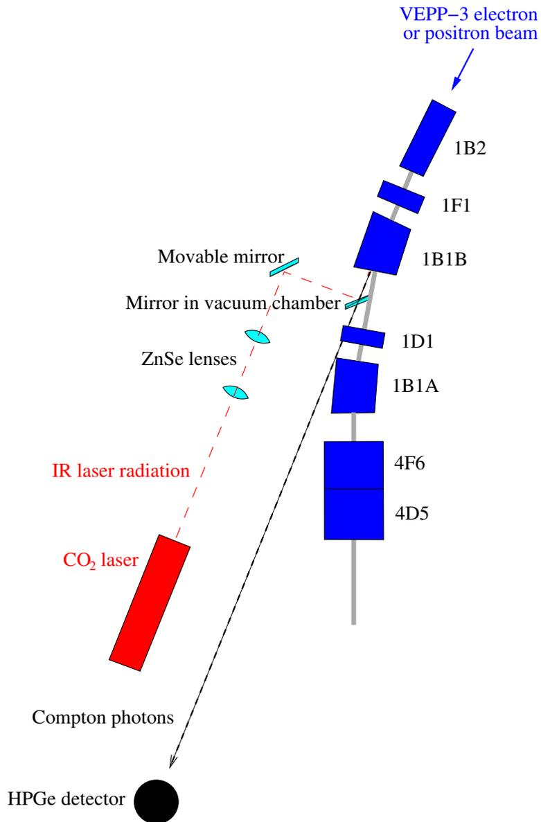
**Figure 2.** Layout of the VEPP-3 beam energy measurement system.
