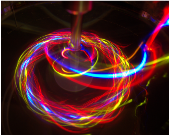
FIG. 55 Long exposure photograph of several finite Stokes number particles moving in the laminar flow of a stirred tank. All particles start in a chaotic flow region but are eventually attracted into a KAM tube where they execute helical trajectories. Photo from Wang, Stewart & Metcalfe.
