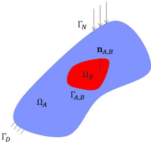
Fig. 2: XFEM two-phase problem model.
