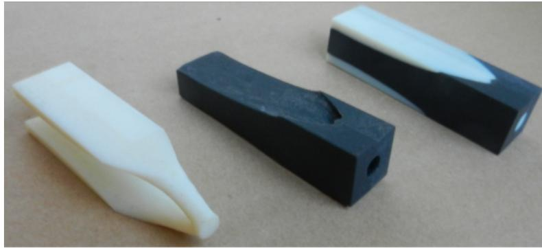
Fig. 21: LSM-XFEM optimized two-phase design for  $E_B = 0.1E_A$  realized by 3D printing.
