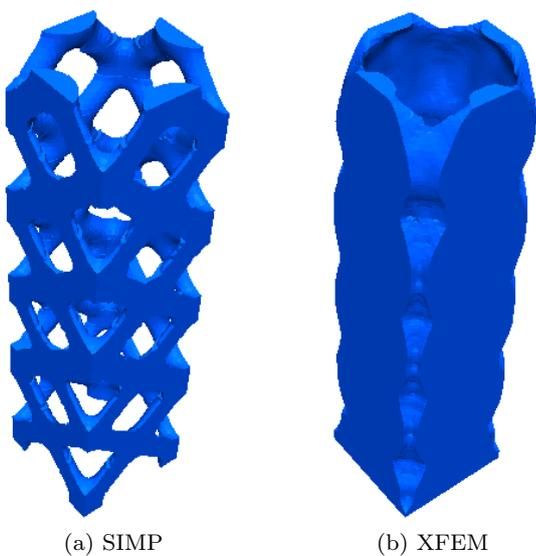
Fig. 17: Topology design with a larger smoothing radius.
