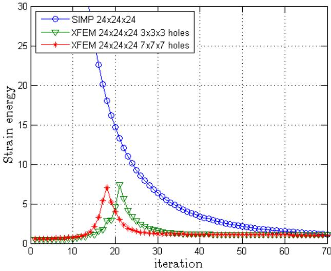
Fig. 11: Convergence plot for the cube with a center load problem.
