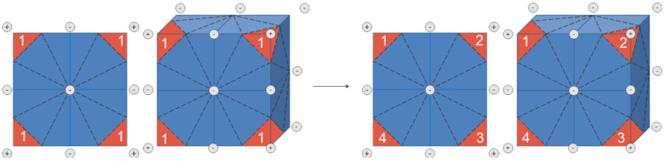
Fig. 5: Distribution of the enrichment functions after the application of the enrichment strategy.
