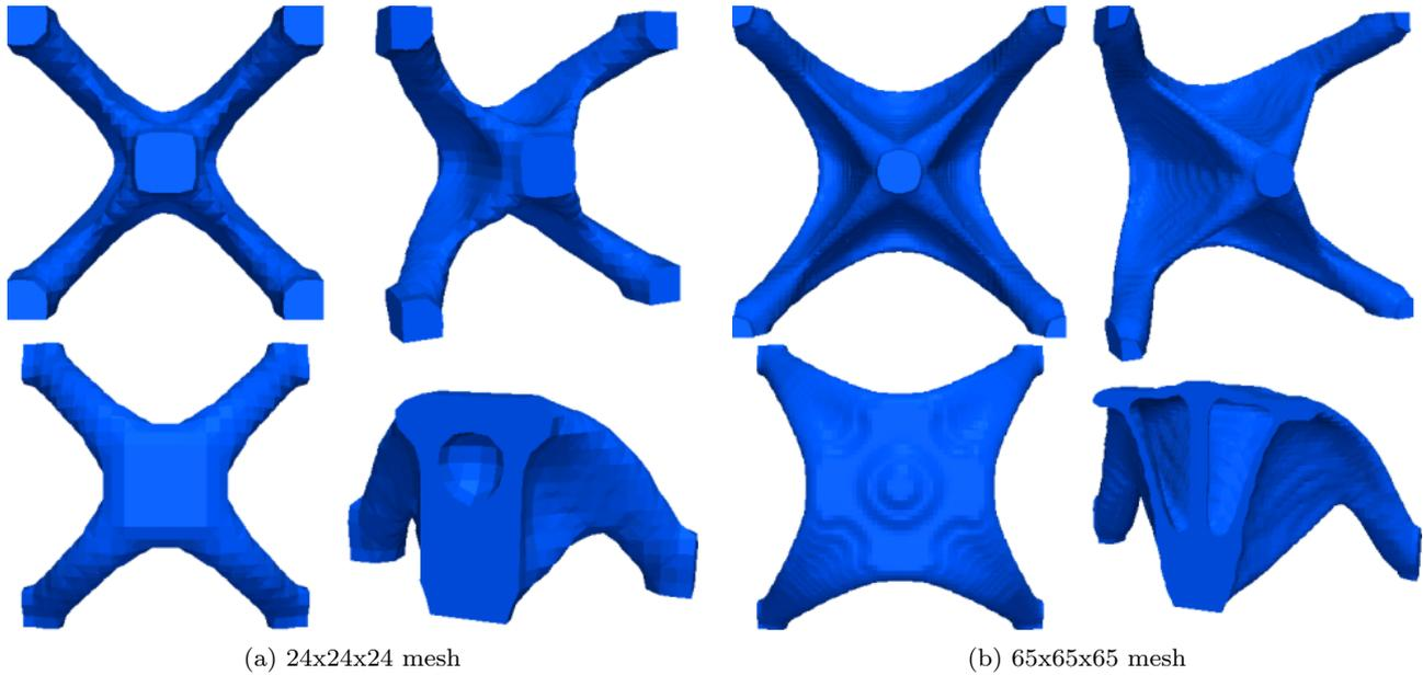
Fig. 7: Cube with center load SIMP topology designs. Clockwise: Bottom, Side, Top, and Clip views.
