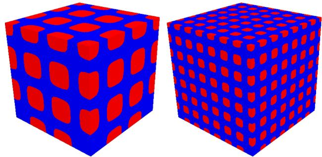
Fig. 9: Initial level set configurations for the cube with a center load problem.
