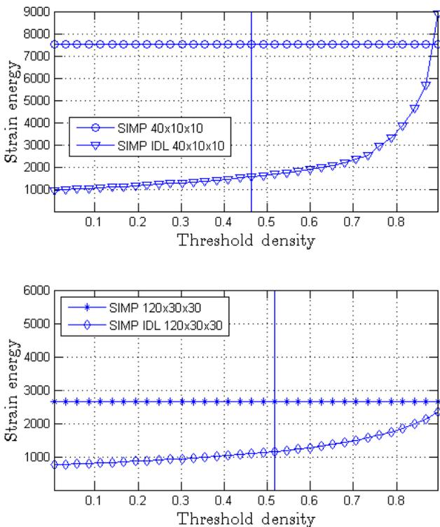
Fig. 16: SIMP-IDL post-processing for the building under torsion problem. The vertical line marks  $\rho_T = 0.46$ , at which the volume constraint is satisfied for both meshes.
