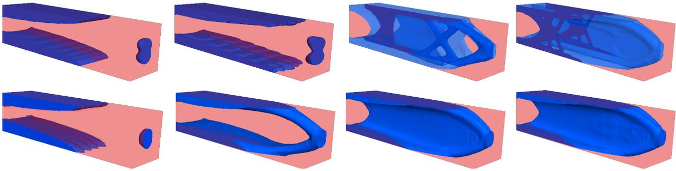
Fig. 20: Two-phase topology optimization using SIMP and XFEM. First row shows the SIMP results, second row, XFEM. Density ratios are from left to right  $E_B = 0.5E_A$ ,  $E_B = 0.1E_A$ ,  $E_B = 0.01E_A$ ,  $E_B$  is void.
