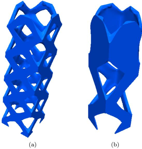
Fig. 18: Cuboid under torsion problem with a perimeter constraint: (a) XFEM restarted from SIMP and (b) XFEM restarted from XFEM.
