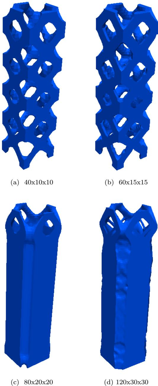
Fig. 13: Cuboid under torsion results with SIMP.  $p = 3$ ,  $r_\rho = 1.6$  of the element edge length,  $\beta = 0$ .
