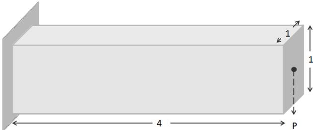
Fig. 19: Initial setup for the long cantilever beam two-phase problem.
