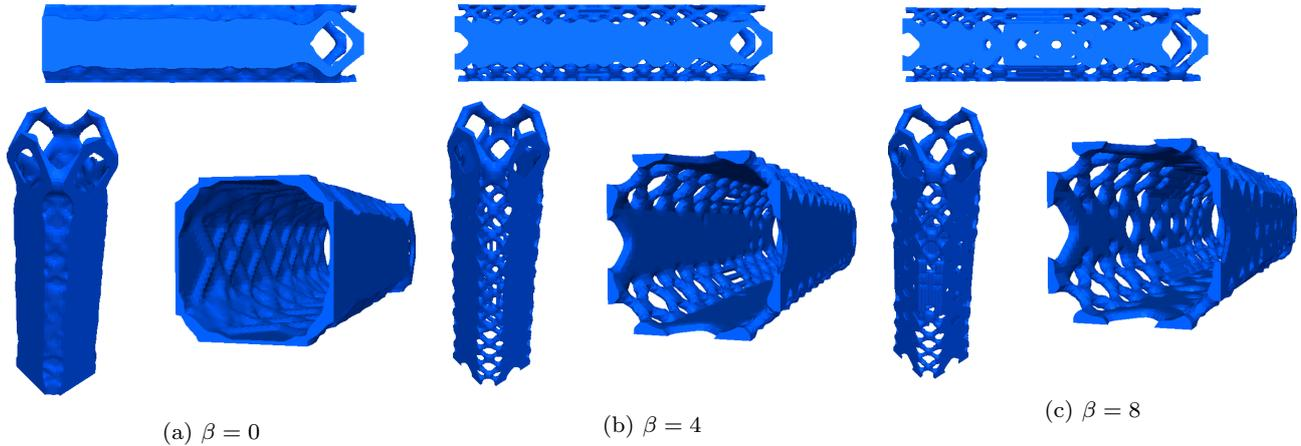
Fig. 15: Density isovolumes of 0.35 for the three step SIMP results.
