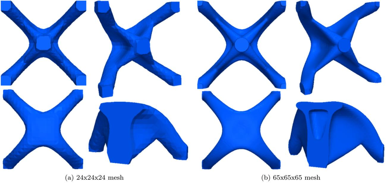
Fig. 10: Cube with center load XFEM topology designs. Clockwise: Bottom, Side, Top, and Clip views.
