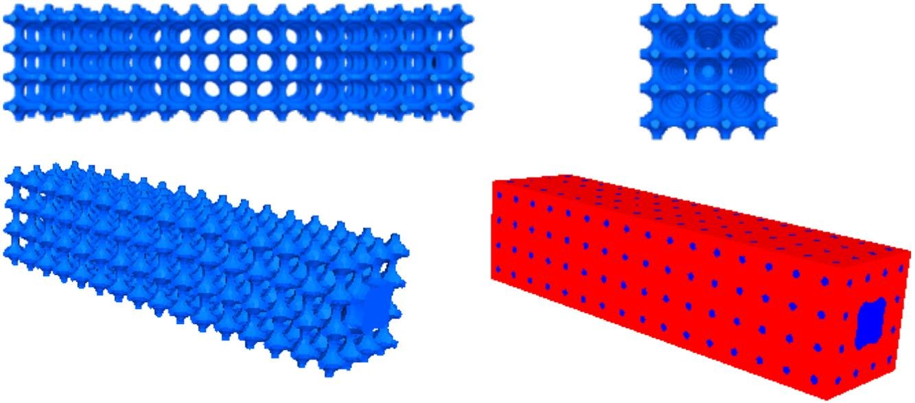
Fig. 1: Initial design with array of spherical inclusions for the cantilever beam example of Section 6.3.
