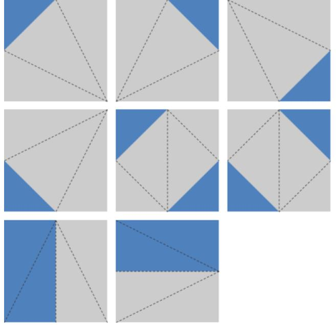
Fig. 3: Intersection pattern for a two-dimensional QUAD4 element.
