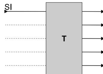
FIG. 2: A nonclassical input state (SI) is combined with a classical  $N-1$ -mode vacuum state (dotted lines). In general, the output state shows multipartite entanglement.
