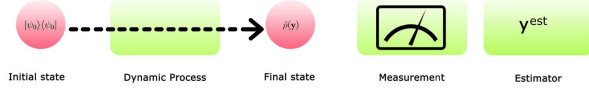
FIG. 1: Scheme of quantum parameter estimation. The final state \hat{\rho}(\mathbf{y}) , evolved from a known initial state allowed by quantum mechanics, carries about the parameter vector characterizing dynamical process, and \mathbf{y}^{est} is obtained from the measurement results performed on the final state.
