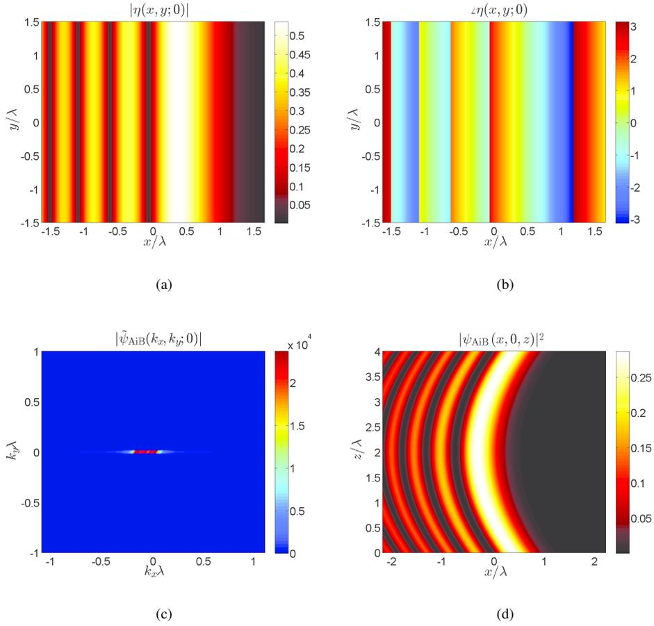
Fig. 3: Generation of a “delayed-start” accelerating beam from a plane-wave. The amplitude and phase of the direct space metasurface function at  $z = 0$  are plotted in (a) and (b), respectively. The  $k$ -space representation of the generated delayed-start Airy beam is plotted in (c) and the intensity profile of the beam in the  $x-z$  plane is plotted in (d). The beam starts its curvature towards the positive  $x$ -axis at  $z = 2\lambda$ .
