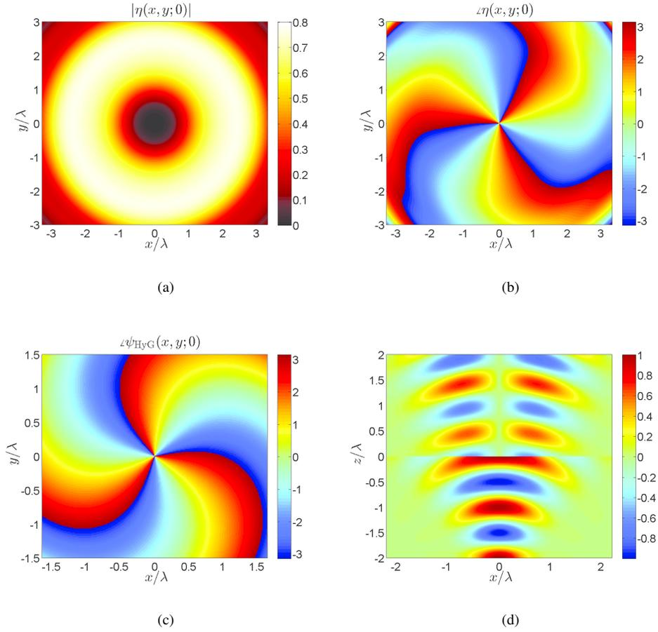
Fig. 2: Generation of a hypergeometric-Gaussian beam from an ordinary Gaussian beam. The amplitude and phase of the direct space metasurface function at  $z = 0$  are plotted in (a) and (b). The phase of the transmitted field is plotted in (c) showing a vorticity corresponding to a topological charge  $m = 3$ . A propagation plot in the  $y = 0$  plane is presented in (d) showing the incident Gaussian beam and the transmitted vortex hypergeometric-Gaussian beam.
