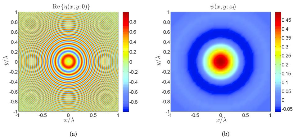
Fig. 5: Holographic repetition from a plane-wave. The direct space metasurface function at  $z = 0$  is plotted in (a) and the reconstructed field at  $z = 300\lambda$  due to a normally incident plane-wave is plotted in (b). The metasurface function bears an uncanny resemblance to a Fresnel lens.
