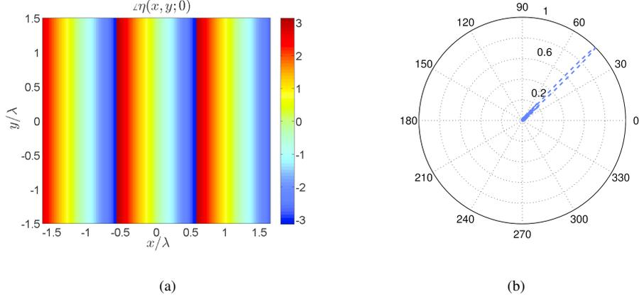
Fig. 4: Generation of a tilted pencil beam from a plane wave. The phase function of the metasurface to generate the tilted pencil beam at angle  $\theta_t = \pi/4$  is depicted in (a). The equivalent directivity of the metasurface is plotted in (b).
