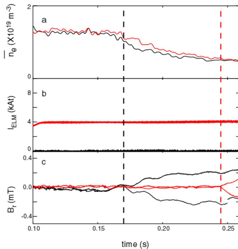
**Figure 11** Time traces of a) line average density ( $\bar{n}_e$ ), b) the current in the ELM coils ( $I_{\text{ELM}}$ ) and c) the radial field component of the magnetic field determined from an array of saddle coils.
