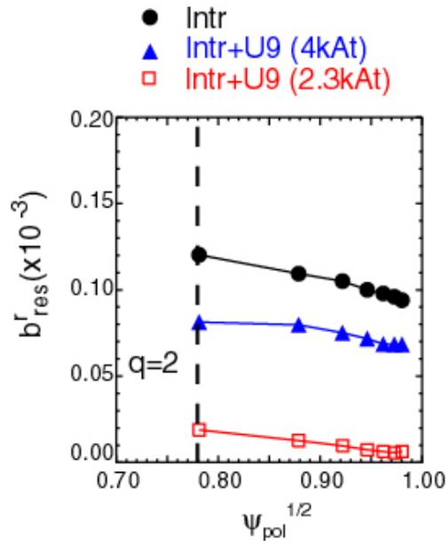
**Figure 16** Calculations in the vacuum approximation of the normalised resonant component of the applied field ( $b_{res}^r$ ) for the intrinsic only (circle), intrinsic plus empirically determined error field correction from the ELM coils (triangle) and the intrinsic plus optimum predicted correction (square). The vertical dashed line shows the location of the  $q=2$  surface.
