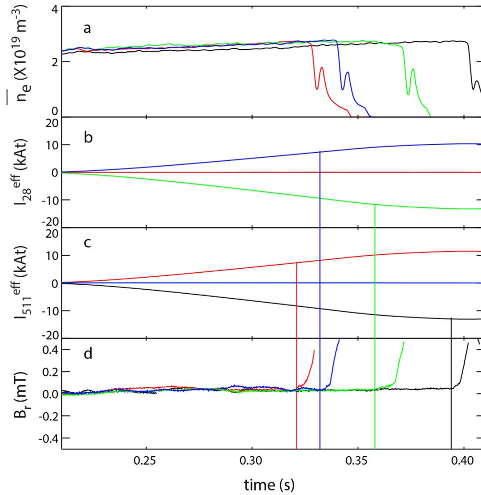
**Figure 4** Time traces for a series of shots with  $I_p=400$  kA, with  $I_{p5}/I_{p4}=1.8$  of a) line average density ( $\bar{n}_e$ ), the effective current in the EFCC pair b) 2-8 ( $I_{28}^{\text{eff}}$ ) and c) 5-11 ( $I_{511}^{\text{eff}}$ ) and d) the radial field component of the magnetic field determined from an array of saddle coils.
