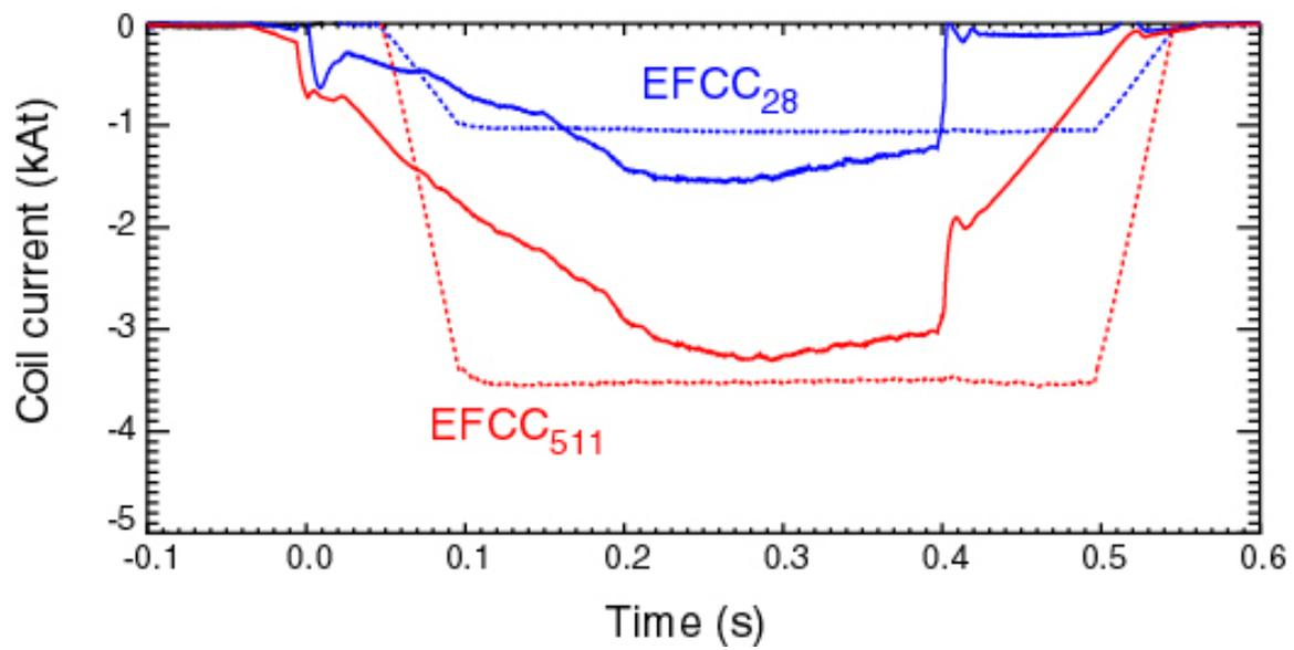
**Figure 8** Example of time traces of the current waveforms in the EFCC for the old (dashed) and new (solid) correction waveforms.
