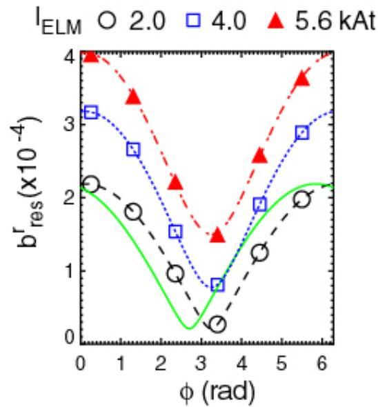
**Figure 17** The effect of changing the amplitude and phase angle of the correction field from the ELM coils on the normalised resonant component of the applied field ( $b^r_{res}$ ). The dashed curves are a fit to the intrinsic and applied field described in the text. The solid curve is the results of the fit to the empirically critical density.
