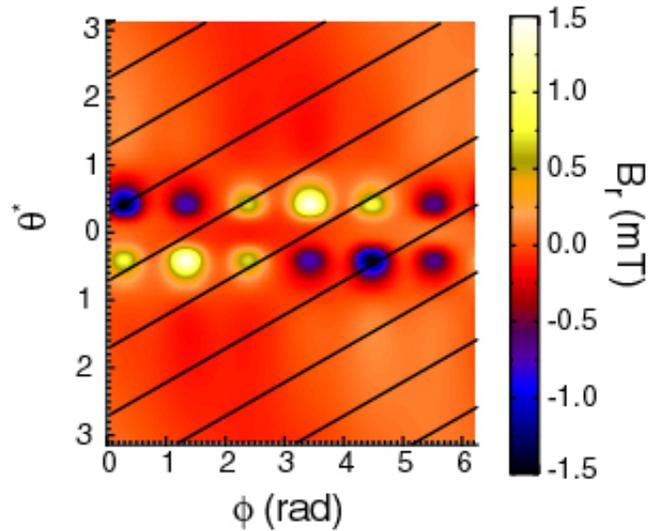
**Figure 10** Plot of the component of the magnetic perturbation (vacuum approximation) perpendicular to the equilibrium flux surfaces as a function of toroidal angle ( $\phi$ ) and the poloidal angle in a straight field line co-ordinate system ( $\theta^*$ ) on the  $q=2$  flux surface for discharges with  $I_p = 600$  kA for a configurations designed to reduce the  $n=1$  component of the intrinsic error field. The solid lines show the equilibrium field lines at the  $q=2$  surface.
