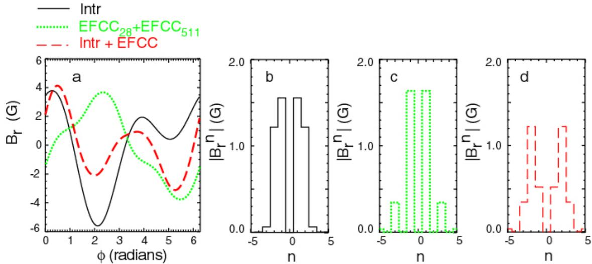
**Figure 13** a) The radial field at the location of the  $q=2$  surface at the low field side midplane, calculated using vacuum modelling due to the intrinsic error field only (solid), EFCCs only (dotted) and corrected field (dashed). The toroidal components of the radial field for b) the intrinsic error field, c) the EFCCs and d) the corrected field.
