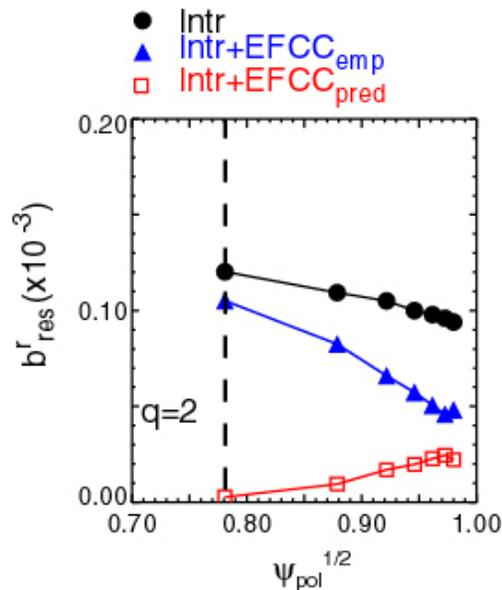
**Figure 14** Calculations in the vacuum approximation of the normalised resonant component of the applied field ( $b_{res}^r$ ) for the  $n=1$  components of the intrinsic only (circle), intrinsic plus empirically determined error field correction from the EFCCs (triangle) and the intrinsic plus optimum predicted correction (square). The vertical dashed line shows the location of the  $q=2$  surface.
