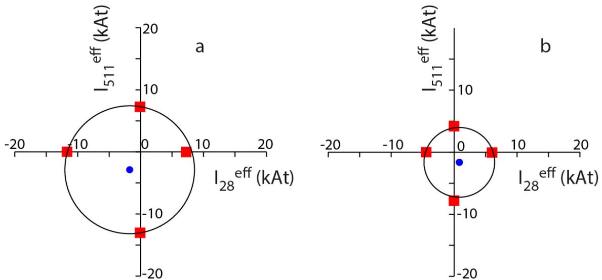
**Figure 6** The error field coil currents required to form a locked mode for an equilibrium with  $I_p = 400$  kA with a)  $I_{P5}/I_{P4} = 1.8$  and b)  $I_{P5}/I_{P4} = 0.25$ .
