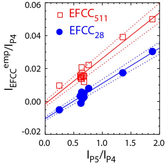
**Figure 7** The empirically derived error field correction current ( $I_{EFCC}$ ) expressed as a fraction of the current in the P4 coils ( $I_{P4}$ ) versus the ratio of currents in P5 over P4 ( $I_{P5}/I_{P4}$ ) for the 2-8 (circle) and 5-11 (square) EFCC pairs. The solid lines show the results of a linear fit to the data and the dotted lines the  $\pm 1\sigma$  contours.
