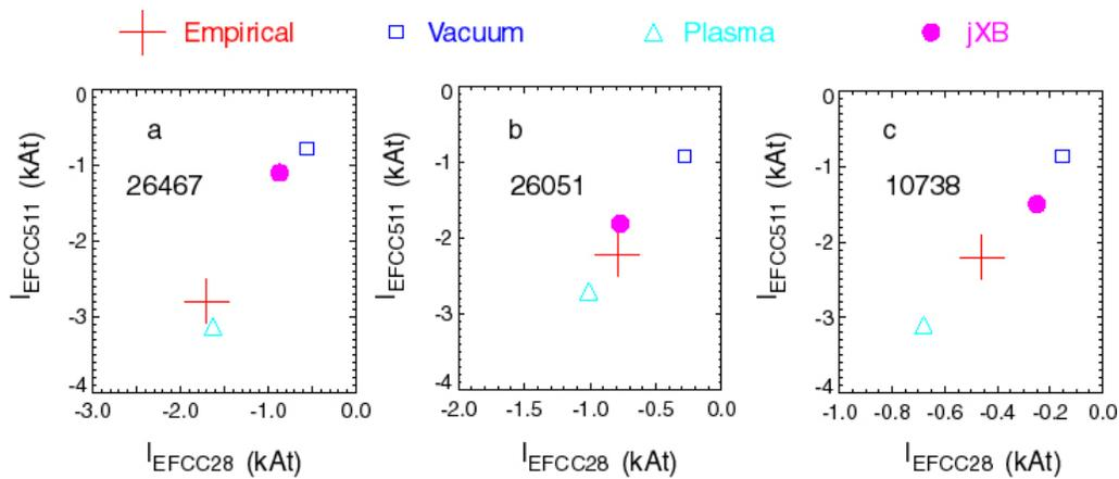
**Figure 18** Coil in the EFCC correction coils found to empirically correct the intrinsic error field correction (cross), to minimise the  $n=1$   $m=2$  radial field component at the  $q=2$  surface using the vacuum approximation (square) or taking into account the plasma response (triangle) and minimising the  $jxB$  torque on the plasma (circle) for shots a) 26467, b) 26051 and c) 10738.
