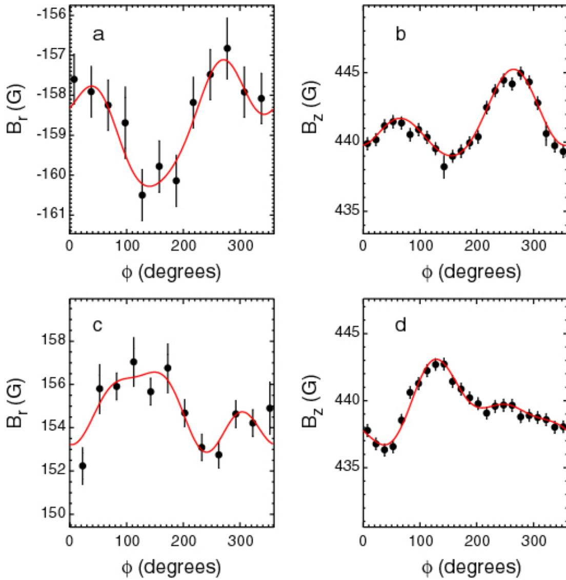
**Figure 2** Measurements of the radial ( $B_r$ ) and vertical ( $B_z$ ) magnetic field as a function of toroidal angle ( $\phi$ ) due to a flat top current of -3.5 kA (-80.5 kAt) in the a),b) upper and c),d) lower P4 coils.
