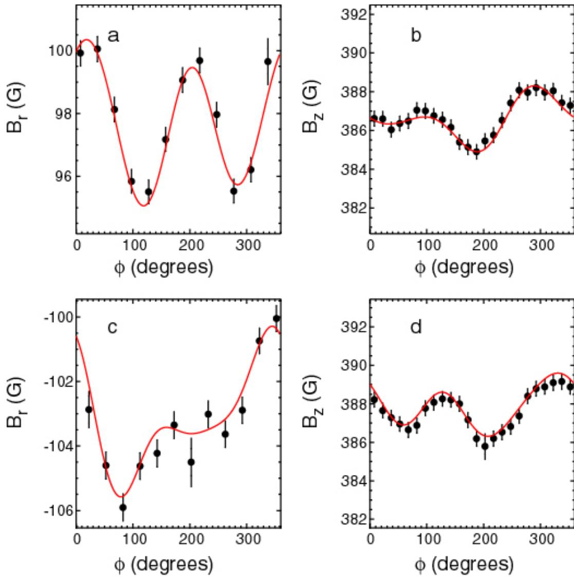
**Figure 3** Measurements of the radial ( $B_r$ ) and vertical ( $B_z$ ) magnetic field as a function of toroidal angle ( $\phi$ ) due to a flat top current of -3.5 kA (-80.5 kAt) in the a),b) upper and c),d) lower P5 coils.
