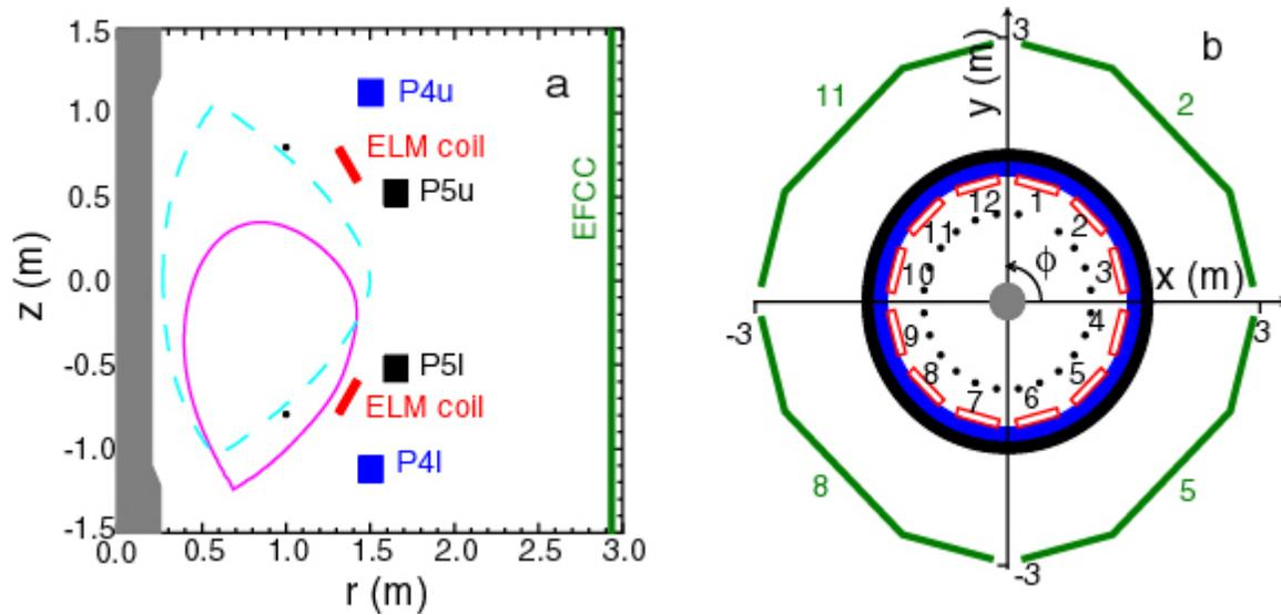
**Figure 1** Location of the poloidal field coils (P4 and P5), the external error field correction coils (EFCC) and internal ELM coils in a) the poloidal cross section and b) the plan view on which are shown the definition of the sector numbers and the toroidal angle ( $\phi$ ). The dots in a) and b) show the location of the Hall probe used to measure the field due to the P4 and P5.
