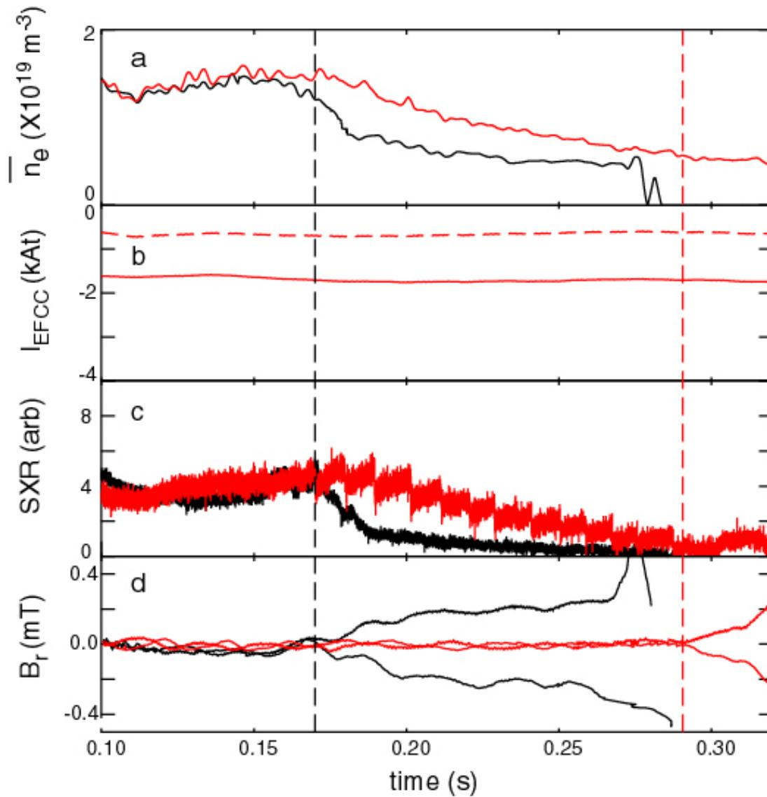
**Figure 9** Time traces of a) line average density ( $\bar{n}_e$ ), b) the effective current in the 2-8 (dashed) and 5-11 (solid) EFCC pairs c) the soft X-ray signal from a core viewing channel and d) the radial field component of the magnetic field determined from an array of saddle coils for a shot without (black) and with (red) error field correction.
