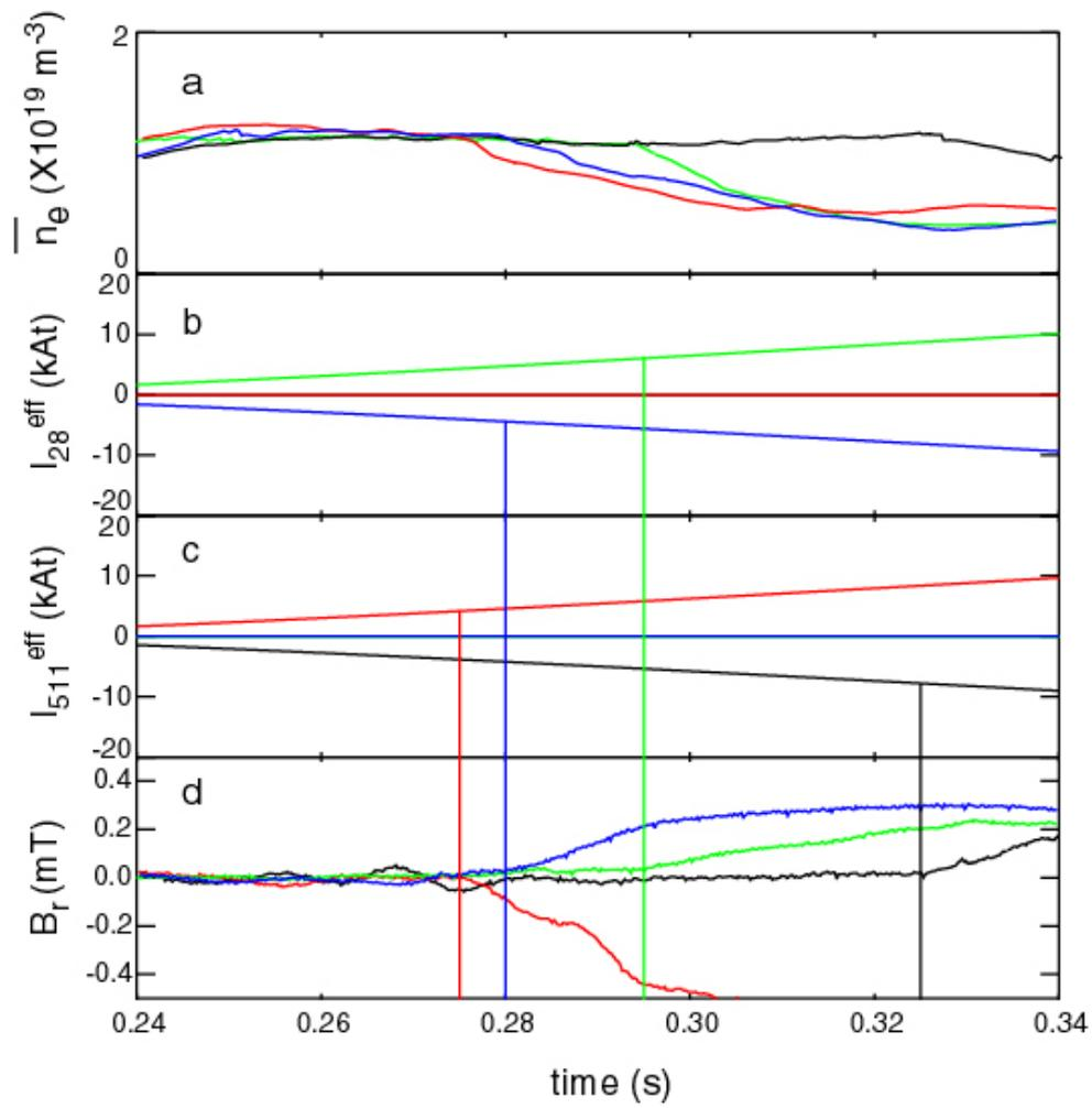
**Figure 5** Time traces for a series of shots with  $I_p=400$  kA, with  $I_{p5}/I_{p4}=0.25$  of a) line average density ( $\bar{n}_e$ ), the effective current in the EFCC pair b) 2-8 ( $I_{28}^{\text{eff}}$ ) and c) 5-11 ( $I_{511}^{\text{eff}}$ ) and d) the radial field component of the magnetic field determined from an array of saddle coils.
