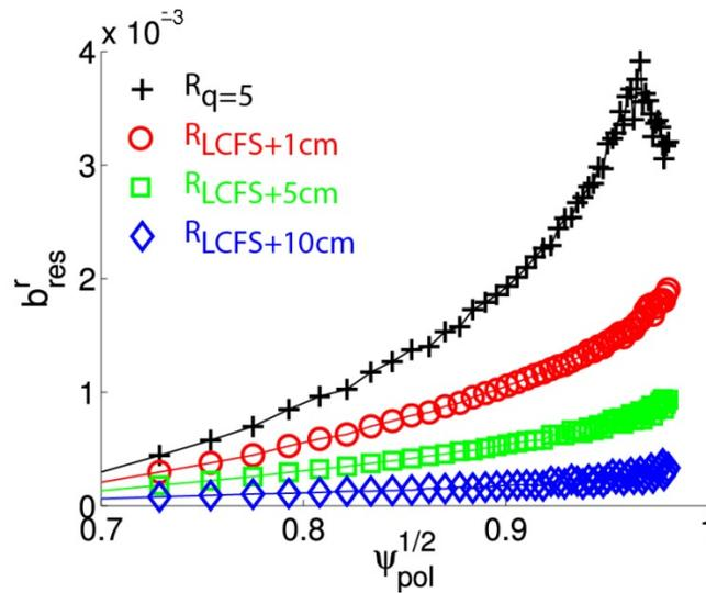
**Figure 8** Radial profile of the normalised resonant component of the applied field ( $b_{res}^r$ ) for 12 equally space filaments each carrying 200 A located inside the LCFS at the  $q_{95}=5$  surface (crosses) and a distance of 1 (circles) 5 (squares) and 10 cm (diamonds) outside the LCFS.
