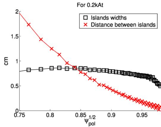
**Figure 7** Calculated island size (squares) and distance between islands (crosses) calculated in the vacuum approximation assuming 12 equally space filaments, each carrying 200 A, located at the  $q_{95}=5$  surface.
