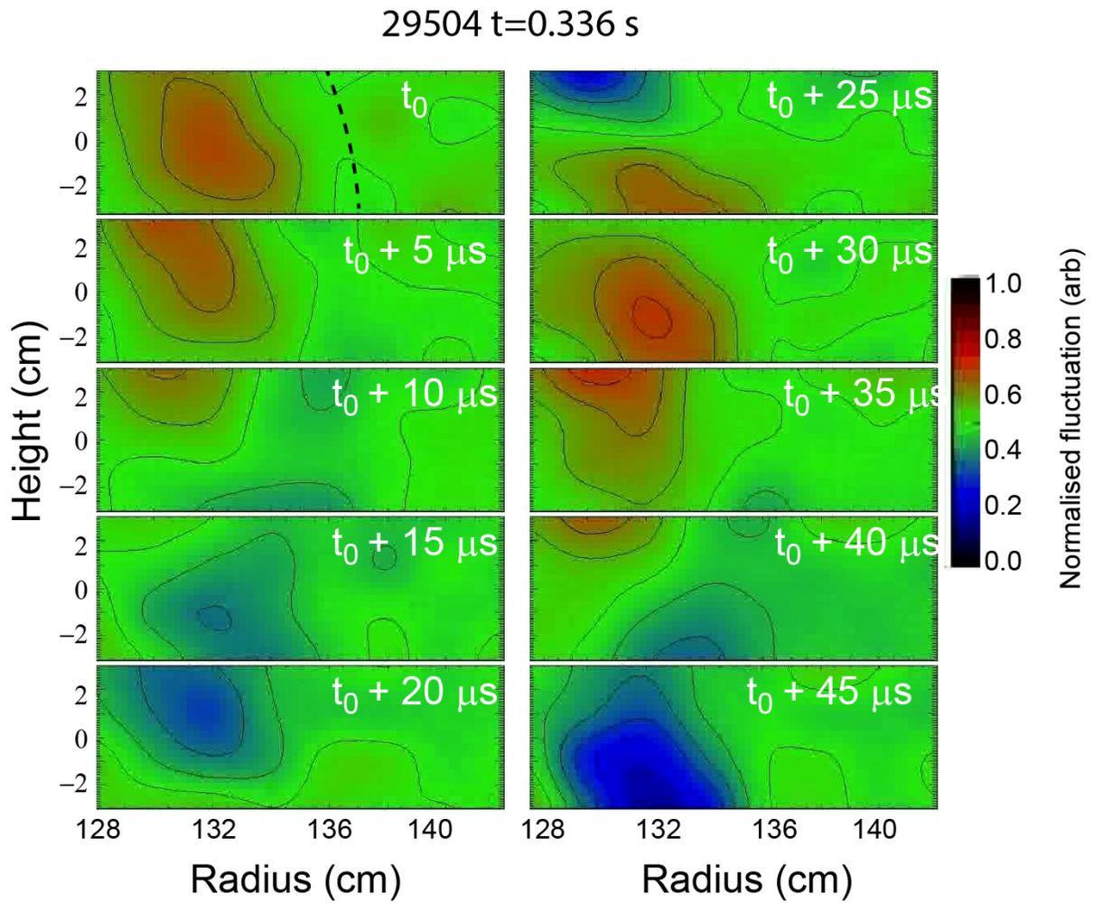
**Figure 4** Turbulence imaging of the plasma edge during the pre-cursor stage leading up to a type I ELM crash on MAST using a Beam Emission Spectroscopy system. The frames shown are separated in time by  $5\mu\text{s}$  relative to a notional time ( $t_0$ ), which is  $\sim 100\mu\text{s}$  before the ELM crash. The dotted curve in the first frame shows the location of the last closed flux surface.
