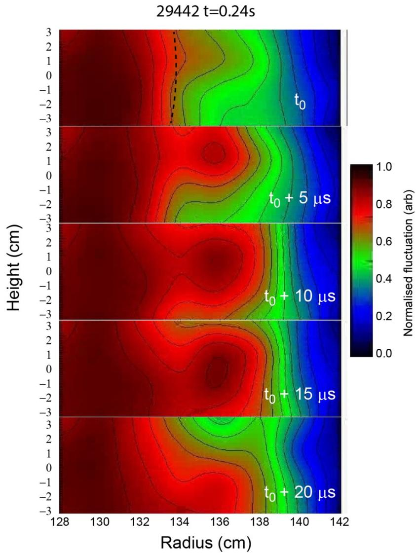
**Figure 3** Turbulence imaging of the plasma edge during an ELM crash on MAST using a Beam Emission Spectroscopy system. The frames shown are separated in time by  $5\mu s$  relative to a notional crash time ( $t_0$ ). The dotted curve in the first frame shows the location of the last closed flux surface.
