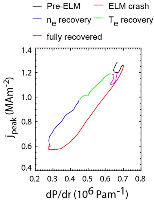
**Figure 1** The peak edge current ( $j_{\text{peak}}$ ) vs the radial pressure gradient ( $dP/dr$ ) calculated using the CLISTE equilibrium code as a function of time during an inter-ELM period on ASDEX Upgrade.
