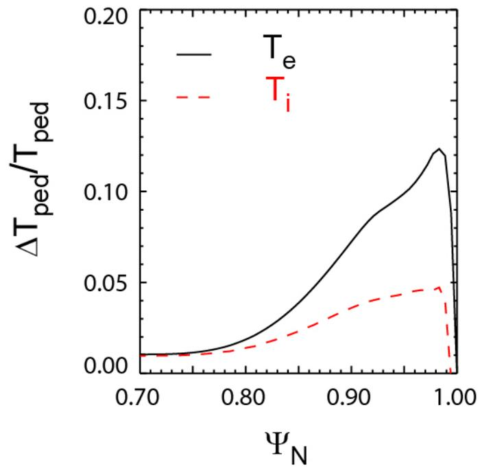
**Figure 9** JOREK simulations of the changes in the electron (solid) and ion temperature profiles due to an ELM in JET normalised to the temperature before the ELM.
