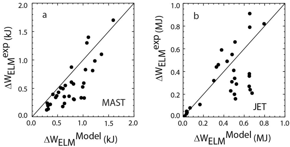
**Figure 5** Measured ELM energy loss ( $\Delta W_{\text{ELM}}^{\text{exp}}$ ) versus the ELM energy loss calculated using a “leaky hosepipe” model ( $\Delta W_{\text{ELM}}^{\text{model}}$ ) for a) MAST and b) JET.
