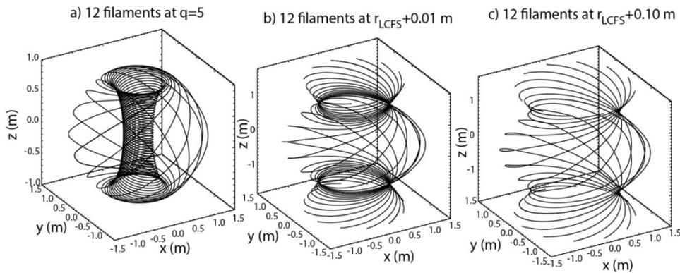
**Figure 6** Simulation of 12 equal toroidally spaced current carrying filaments located a) inside the LCFS on the  $q=5$  surface, b) 1 cm and c) 10 cm outside the LCFS for a MAST like plasma in a connected double null magnetic configuration.
