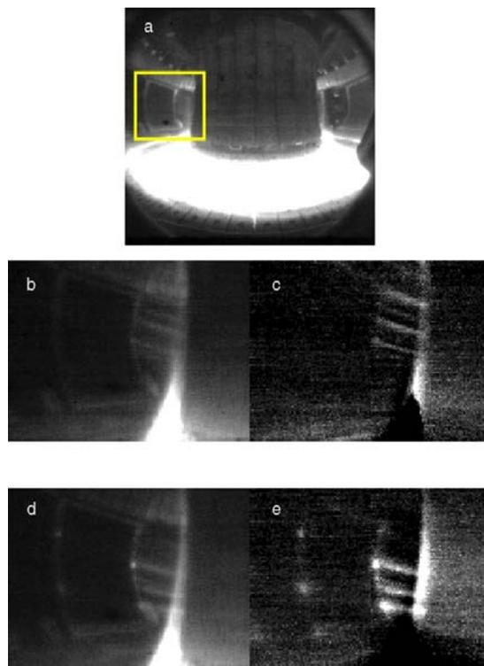
**Figure 2** Visible images obtained on ASDEX Upgrade. a) full view of the plasma with the region of fast acquisition shown as a box. b) image obtained during the start of the rise time of the target  $D_\alpha$  due to an ELM and d) an image obtained 50  $\mu\text{s}$  later during the same ELM. c) and e) are background subtracted versions of b and d respectively.
