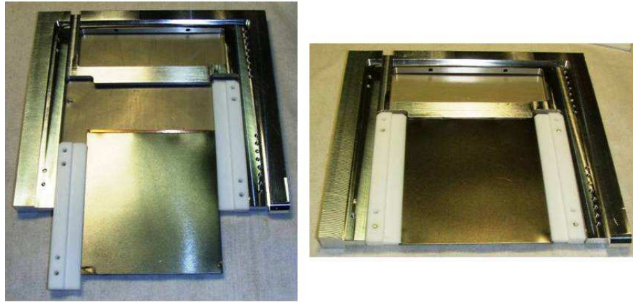
Figure 8. The Aluminium holder and a blade (substrate coated with ^{10}\text{B}_4\text{C} both sides) inserted.
