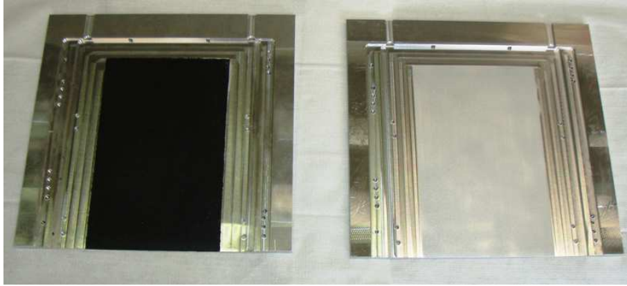
Figure 19. A cassette V2 coated and un-coated with ^{10}\text{B} painting.
