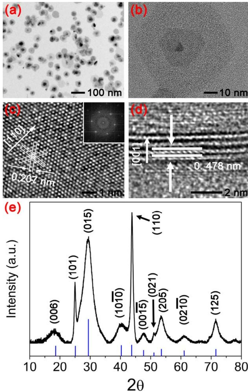
**Figure 1.** (a) Representative TEM image of the PVP-protected  $\text{Bi}_2\text{Se}_3$  nanoplates (NPs), and (b) a magnified image showing a terraced 2-D structure of the NPs. (c,d) High-resolution TEM image of the as-prepared PVP-protected  $\text{Bi}_2\text{Se}_3$  NPs in (c) horizontal plane and (d) in thickness direction. (e) XRD image of the as-prepared PVP-protected  $\text{Bi}_2\text{Se}_3$  NPs. The blue lines are the peaks of bulk  $\text{Bi}_2\text{Se}_3$ .
