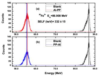
FIG. 2 (color online). Geometry dependent (forward and back) spectra, showing the differential surface energy loss field (SELF) effect of the bilayer targets (a) Al-PP and (b) PP-Al.
