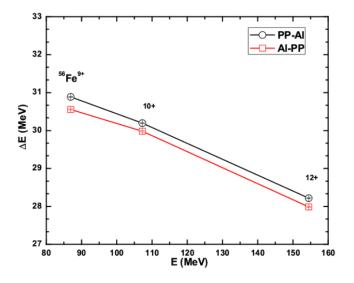
FIG. 3 (color online). Beam energy dependent energy loss in Al-PP and PP-Al bilayer targets illustrating the SELF difference effect.
