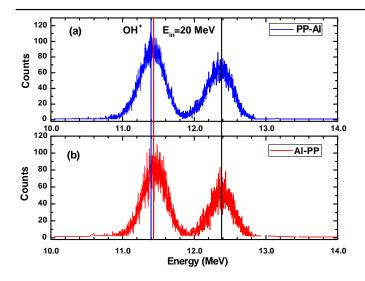
FIG. 4 (color online). Geometry dependent (forward and backward) energy loss spectra of the bilayer targets (a) PP-Al and (b) Al-PP for the molecular Coulomb explosion of  $OH^+$  ion.
