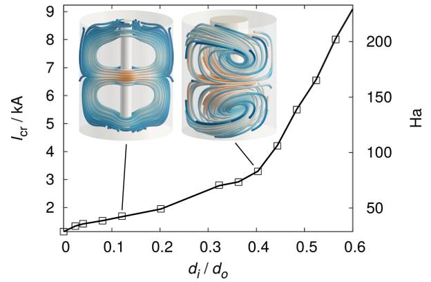
Figure 8: Critical current for an electrode with a bore in the middle ( $d_o = 248 \text{ mm}$ ,  $h = 300 \text{ mm}$ , Na).
