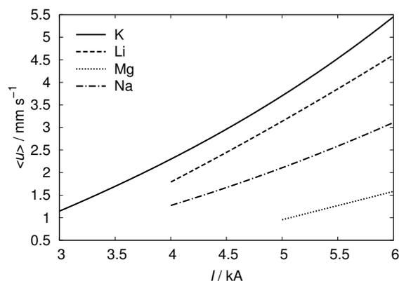
Figure 5: Mean velocity of the saturated TI for different liquid metals in dependence of the applied current.
