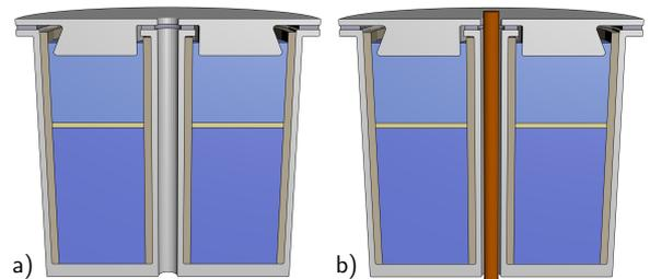
Figure 9: Providing the liquid metal battery with a bore or returning the current are effective ways to avoid the TI.
