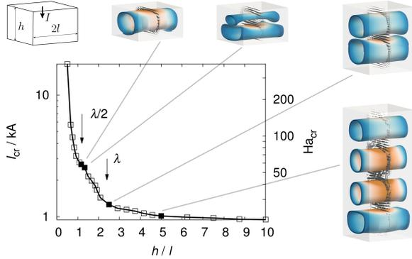
Figure 7: Critical current (Na) and Hartmann number for onset of the TI in dependence of the aspect ratio. Simulations were carried out with a cuboid geometry with the dimensions  $96 \times 96 \times h \text{ mm}^3$ .
