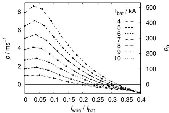
Figure 10: Growth rate of the TI in a liquid metal battery electrode with a return current through a bore of  $d_i = 30$  mm ( $d_o = 248$  mm,  $h = 300$  mm, Na).
