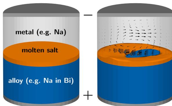
Figure 1: Sketch of a liquid metal battery with typical inventory (left). The electrolyte works as ion conductor and separates the two liquid metals. A movement of the fluid, as it may result from magneto-hydrodynamic instabilities, could wipe the electrolyte and lead to a battery failure (right).
