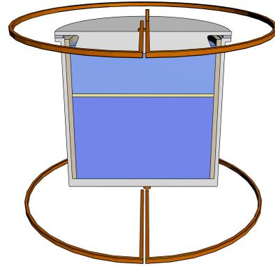
Figure 11: An axial magnetic field produced by a Helmholtz-like coil is an effective way to suppress the TI.
