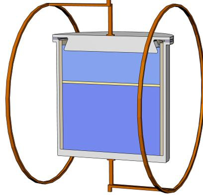
Figure 13: Example of a battery stabilization by a lateral Helmholtz-like coil producing a horizontal magnetic field.
