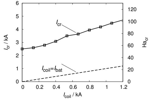
Figure 14: Critical current for onset of the TI in a cuboid Na electrode of the dimensions  $1 \times 1 \times 0.5 \text{ m}^3$ . The stabilizing horizontal magnetic field is produced by a Helmholtz coil with a diameter of 1.2 m.
