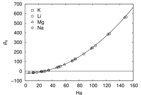
Figure 4: Growth rate of the TI in dependence of the Hartmann number for different liquid metals. The growth rate is normalized to  $\nu/R^2$ .
