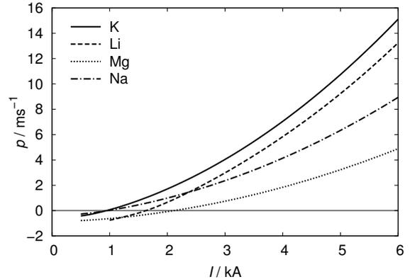
Figure 3: Growth rate of the TI in dependence of the applied current for different anode materials. The critical current corresponds to a growth rate of zero.
