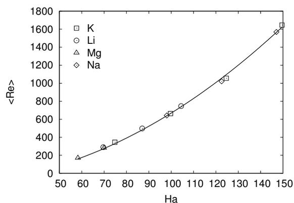
Figure 6: Mean Reynolds number of the saturated TI for different liquid metals in dependence of the Hartmann number.
