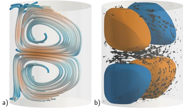
Figure 2: Flow field of the TI (a) in a cylinder filled with liquid Na,  $I = 4$  kA, material parameters taken at  $T = 365$  °C, and contours of the corresponding magnetic field  $b_z$  (b) in the saturated state.
