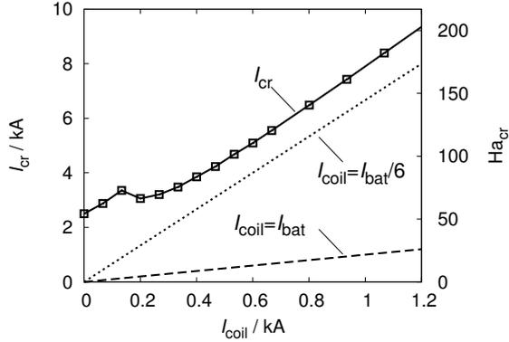
Figure 12: Critical current for onset of the TI in a cuboid Na electrode of the dimensions  $1 \times 1 \times 0.5 \text{ m}^3$  with an external applied magnetic field  $B_z$ , produced by a Helmholtz coil of a diameter of 1.2 m.
