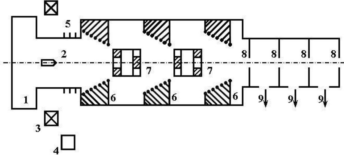
Fig. 1. (1) feeding cassette, (2) particles, (3) pulsed magnetic field coil, (4) electron gun, (5) electrostatic particle acceleration area, (6) - spiral waveguide sections, (7) doublets of quadrupole electrostatic lenses, (8) pulse diaphragms, (9) individual evacuation of buffer cavities.
