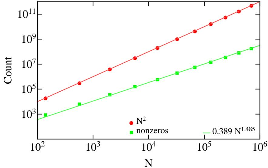
Figure 3: (Color Online) The sparsity of the light-cone Hamiltonian matrix  $H_{\text{LC}}^{(\text{pos})}$ . The horizontal axis is the dimensionality  $N$  of the basis space. The square dots show the number of nonzero matrix elements. A power-law fitting suggests the number of nonzero elements is proportional to  $\sim N^{1.485}$ .
