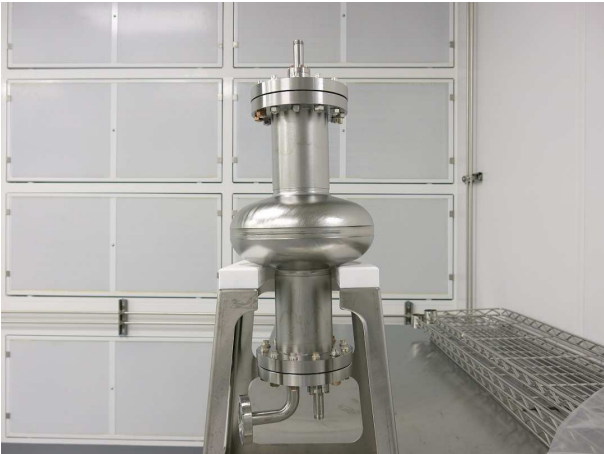
Fig. 6. (color online) The 1.3GHz Tesla-type single-cell cavity doped with Sc
