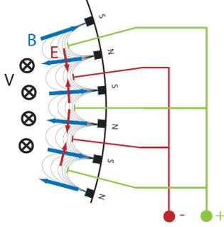
FIG. 5. A cartoon of the flow drive mechanism in MPDX using biased anode-cathode pairs in the cusp field. The torque is proportional to the anode-cathode bias voltage, current and their location in the cusp which determines  $B$
