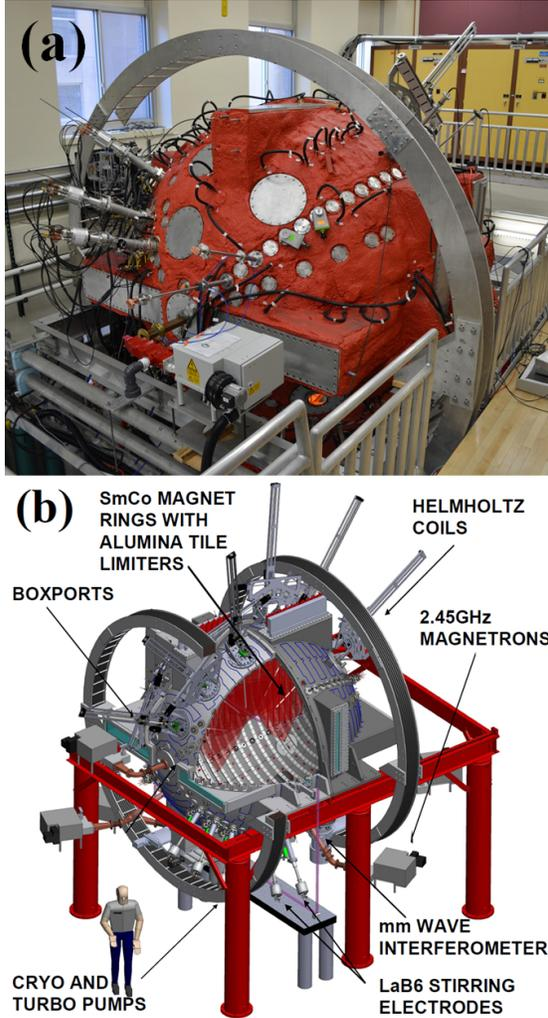
FIG. 1. (a) a picture of MPDX and (b) the various current and planned subsystems labeled.
