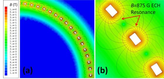
FIG. 3. (a) Poloidal magnetic flux contours for the MPDX (magnetic field lines) and color contours of the magnetic field strength as computed by the MaxwellSV finite element modeling package and (b) a closeup of the cusp. The magnetic field is generated by axisymmetric rows of 4000 G SmCo magnets with alternating polarity. The central dark blue contour shows the region where the magnet-produced field is less than 0.2 gauss and the red contour shows the 875 G ECH resonance surface.
