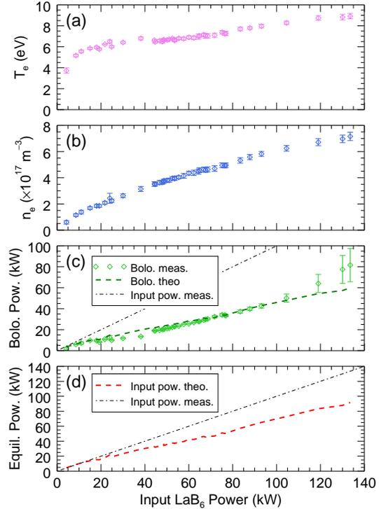
FIG. 8. The scaling of (a)  $T_e$ , (b)  $n_e$  and (c) radiated power measured while varying the input power from 4 - 135 kW into  $6.5 \times 10^{-5}$  Torr helium. The data are used to predict the radiated and equilibrium power required using a confinement a model which is compared to the input power (d) by the LaB<sub>6</sub> cathodes.
