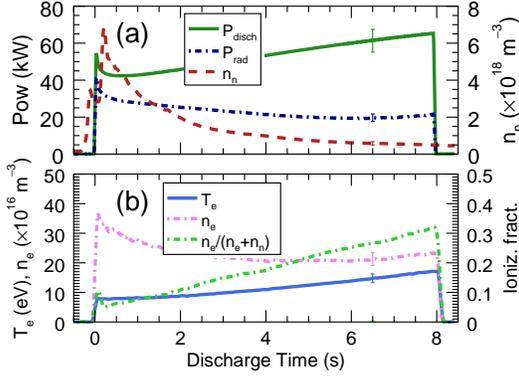
FIG. 6. (a) Time trace of the gas puff, the input power, and the radiated power from the bolometer (b)  $T_e$  measured by a Langmuir probe,  $n_e$  measured by an interferometer normalized to a path length measured by probes, and the calculated ionization fraction  $n_e/(n_n + n_e)$ .
