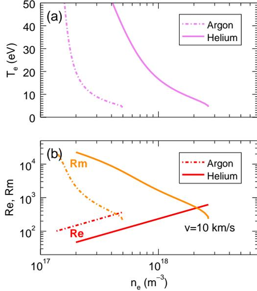
FIG. 11. Plasma parameters calculated using the confinement code described above for an input power of 300 kW and  $v_\phi = 10$  km/s over a scaling of  $n_e$  achieved by varying the fill pressure in Argon (dashed) and Helium (solid). (a) The tradeoff between  $T_e$  and  $n_e$ . (b) The tradeoff between  $Re$  (red) and  $Rm$  (orange). This creates a scaling of magnetic Prandtl number  $0.01 < Pm = Rm/Re < 100$  with the intersections of the lines corresponding to  $Pm = 1$ .
