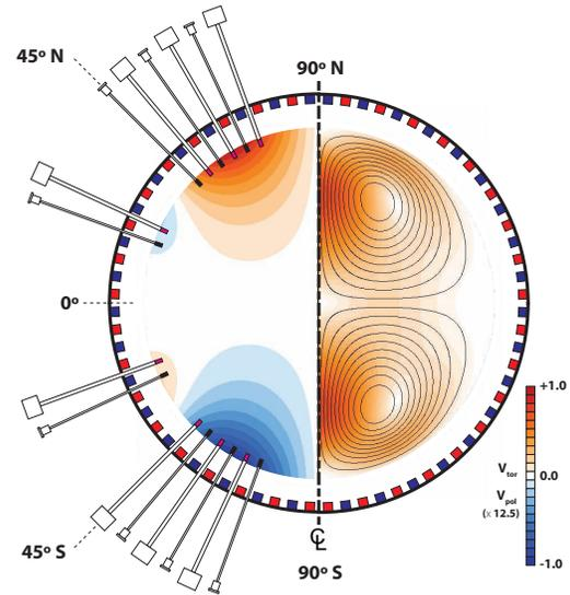
FIG. 13. Numerical simulations of the boundary driven flow with for the flow drive with  $Re = 300$  in a Von Kármán geometry with counter rotating flows in each hemisphere. The poloidal flows (right side) develop self-consistently as a response to the centrifugal forces developing due to toroidal (left) rotation.
