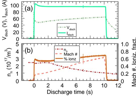
FIG. 9. (a) A time trace of the input voltage, current, and power as measured at the anode and cathode and (b) the toroidal flow  $v_\phi$  measured by a Mach probe, the neutral density measured by a cold cathode gauge and the ionization percentage. As the puffed neutral gas is pumped out, the neutral drag decreases and the plasma spins faster.
