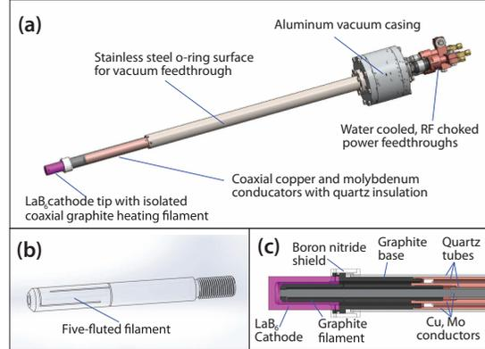
FIG. 4. LaB<sub>6</sub> stirring electrode design. The entire (1.1 meter long) electrode is shown in (a), with detailed views of (b) the graphite heater filament and (c) the LaB<sub>6</sub> tip. Not shown: the linear vacuum feedthrough and garage / gate-valve assembly.
