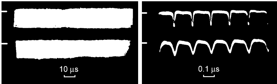
Fig.6. Stable vortex structure in magnetron r_a = 3.2cm ; r_c = 1.0cm ; L = 7cm ; B = 1.5kG ; V = 1.0kV ; p = 1 \times 10^{-5} Torr .
