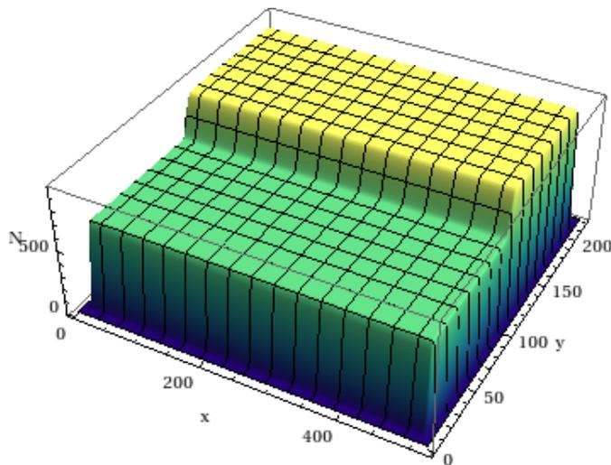
Figure 31: Integrated power spectra of SR Light at the IC due to a real beam of size ( $R_{\text{beam}} = 100\mu\text{m}$ ) -  $X, Y(10\mu\text{m})$ ;  $N(\times 10^{12})$ . (The difference between the profile has been enlarged for clarity)
