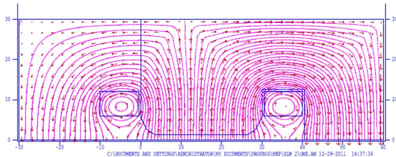
Figure 14: Field map of the dipole face at the edge of the dipole.
