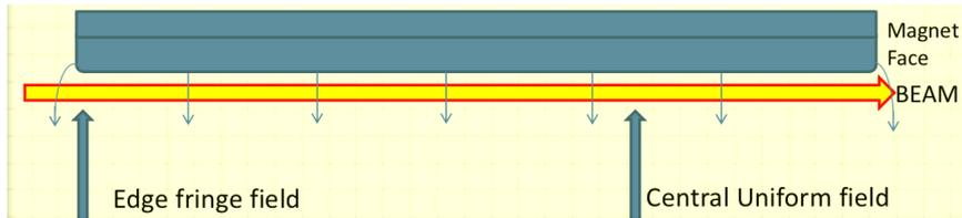
Figure 11: Schematic diagram of the planes at which position the simulation was carried out.
