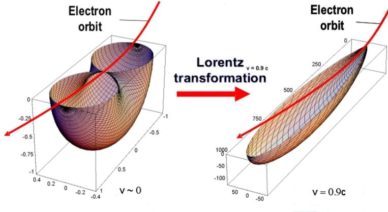
Figure 1: Angular distribution of synchrotron radiation shown for the bottom half of the electron's orbital plane. The left figure is for slow electrons,  $\beta \sim 0$  and the right figure is for highly relativistic electrons,  $\beta \sim 1$ . [1]
