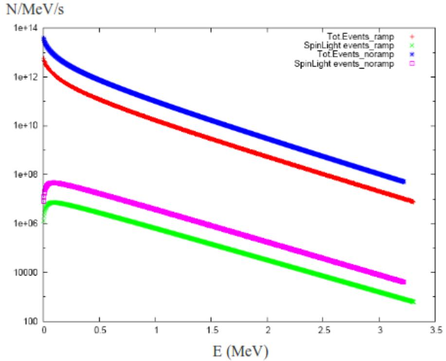
Figure 16: Plot showing the SR - Light (*TotEvents\_ramp*) and Spin - Light (*SpinLightEvents\_ramp*) power spectra with a realistic taper for the dipoles (Power spectra for uniform magnetic field have also been presented as *\_noramp*).
