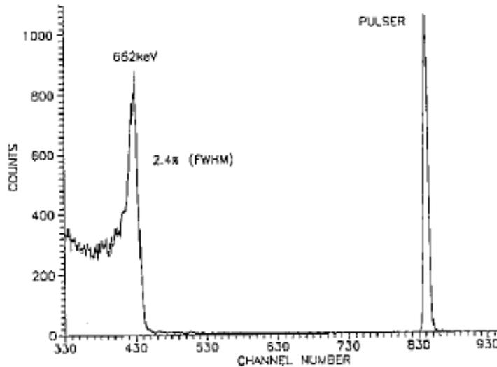
Figure 6: Cs<sup>137</sup>:  $E_i = 1.7\text{kV/cm}$ , pulse height spectrum in 57atm at 295K of xenon,  $E_i = 1.7\text{kV/cm}$  [14].
