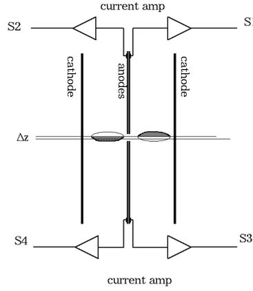
Figure 24: A schematic diagram of signal collection configuration.
