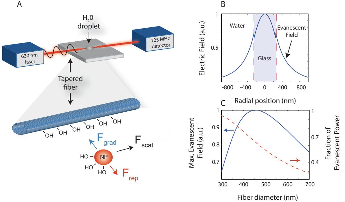
FIG. 1. (a) Experimental setup of the nanofiber tweezer. The surface functionalization of the fiber and nanoparticle (NP) create a repulsive electrostatic force which is opposed by the attractive optical gradient force. (b) Finite element simulation of radial variation in electric field amplitude for a 500 nm nanofiber. (c) Electric field amplitude (left) and fraction of evanescent power (right) as a function of various nanofiber diameters.
