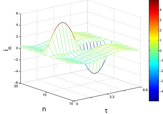
**Fig. 8** Spatiotemporal evolution of a dissipative, period-3 breather during three driver periods, for a SQUID metamaterial with  $N = 30$ ,  $\phi_{dc} = 0$ ,  $\phi_{ac} = 1.2$ ,  $\gamma = 0.001$ ,  $\beta = 1.27$ , and  $T_b = 12.57$ .
