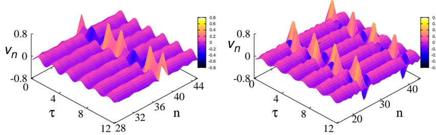
**Fig. 9** Spatiotemporal evolution of dissipative breathers excited spontaneously in weakly disordered rf SQUID metamaterials in 1D during six periods. The voltage amplitude in the Josephson junction of the  $n$ th SQUID  $v_n = d\phi/d\tau$  is plotted on the  $\tau - n$  plane for  $\phi_{dc} = 0$ ,  $\phi_{ac} = 0.03$ ,  $\beta = 1.27$ ,  $\gamma = 0.001$ ,  $\lambda = -0.0014$ ,  $\omega = 3.11$ , and  $N = 50$ . The left and right panels correspond to different configurations of disorder.
