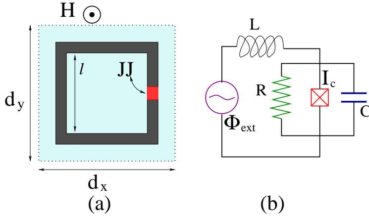
**Fig. 4** (a) Schematic drawing of the unit cell of a SQUID metamaterial with one SQUID per cell. The applied magnetic field  $\mathbf{H}(t)$  is perpendicular to the SQUID plane. (b) The equivalent Resistively and Capacitively Shunted Junction (RCSJ) model for an rf SQUID with one Josephson junction driven by a flux source  $\Phi_{ext}$ .
