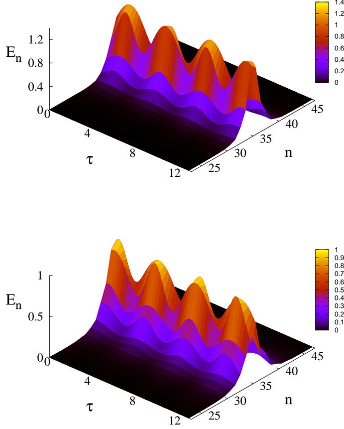
**Fig. 12** Spatiotemporal evolution of the energy density  $E_n$  on the  $n - \tau$  plane during two periods of oscillation for a  $\mathcal{PT}$  metamaterial with  $N = 70$ ,  $N_\ell = 10$ ,  $\gamma = 0.002$ ,  $\lambda'_M = -0.10$ ,  $\lambda_E = \lambda'_E = 0$ , and (upper)  $\lambda_M = -0.17$ ; (lower)  $\lambda_M = -0.21$ . Energy localization at two neighboring sites, one with gain and one with loss, is clearly observed.
