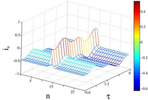
The strong nonlinearity in the SQUIDs manifests itself also with the existence of several simultaneously stable solutions. The multistability of SQUID states implies multistability for possible DB configurations; indeed, by combination of two or more simultaneously stable single SQUID states for the construction of 'trivial breathers', we may generate simultaneously stable DBs [25]. Typical DBs of
