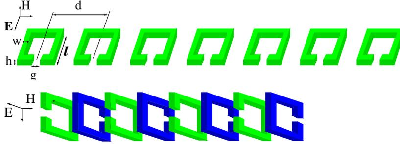
**Fig. 1** Schematic view of a one-dimensional array of split-ring resonators in (upper) the planar geometry; (lower) the axial geometry. The magnetic field is perpendicular to the planes of the rings.
